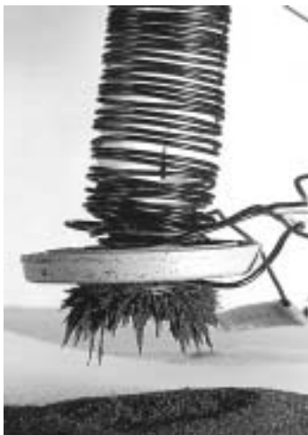
Figure 3 My electromagnet: a long nail that lifts magnetite sand from a pile when its coiled wires are connected to D cells. Photo by Joe Peidle.
