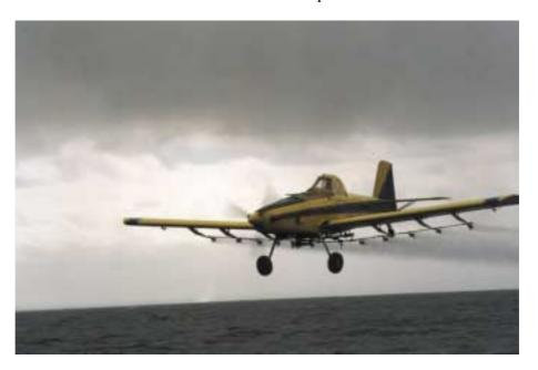
An Air Tractor used in dispersant application operations
