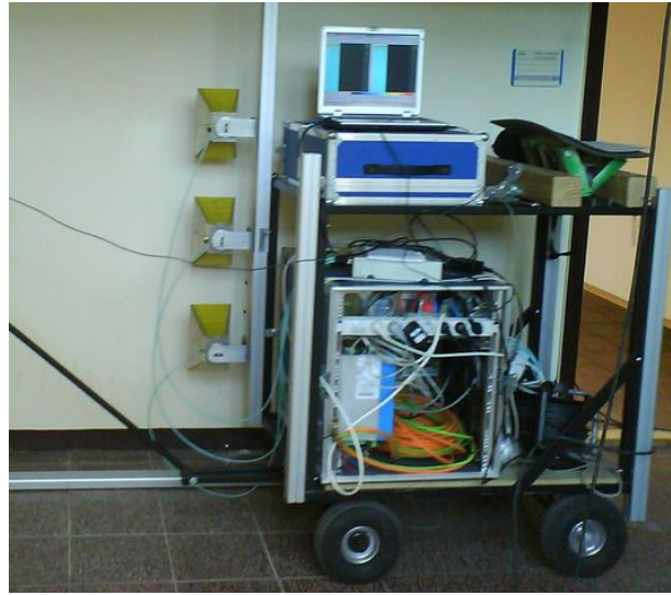
Fig. 4.1.5: Trolley antenna movement - positioner system.
