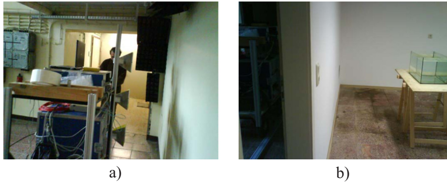
Fig. 4.4.2: SAR measurement. a) Radar system in front of the wall. b) Aquarium filled with water behind the wall.
