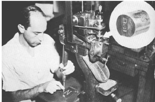
CUTTING THE MATRIX —engraving machine in operation. Operator follows metal template with stylus, as cutter engraves character into die. Inset shows face of die.
