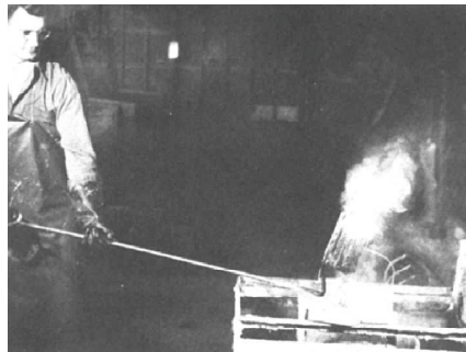
HARDENING BATH —newly pressed slugs are bathed in cyanide at 1600°.
