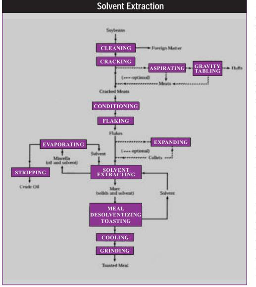
as meats. Often times, the hull fractions from the aspirators are passed over a gravity table to salvage small pieces of meats that are aspirated along with the hulls. There are several advantages for removing the hull: less total volume to process, which means greater extraction output per day and improved protein content of the meal.
