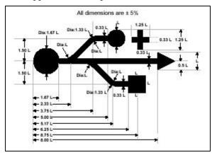
Id be drawn as shown in the USB 2.0 specification, figure  $6.5^2$ . This diagram reproduces the specification figure with the additional plus sign shown with suggested positioning and relative size dimensions. Note that manufacturers should feel free to scale the image as required by their production process in order to fit it on a surface near the PC or host port.
