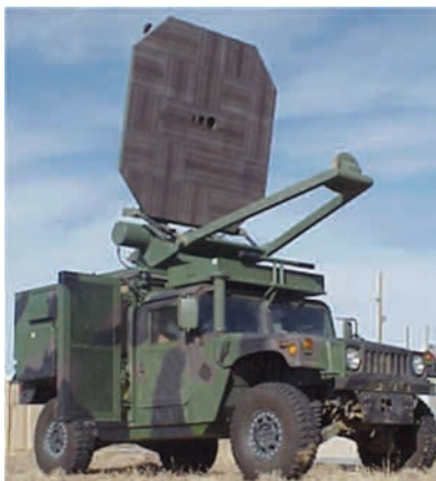
Figure 2. Vehicle Mounted Active Denial System. The sensation causes targeted individuals to repel or retreat. (Photo Courtesy of US Air Force Research Laboratory's Directed Energy Directorate.) [7]
