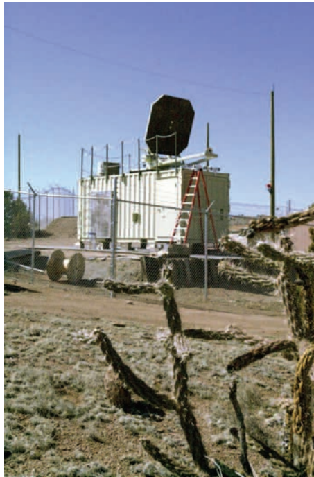
Figure 1. An antenna atop a transportable shelter is the most visible portion of the Active Denial Technology test bed on Kirtland Air Force Base. This technology uses a millimeter wave beam of energy to create an intense heating sensation that repels people without causing permanent injury. (Photo Courtesy of US Air Force Research Laboratory’s Directed Energy Directorate.) [7]
