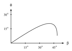
We see that  $\phi$  has a maximum of roughly  $\phi_{\rm max} \approx 20^{\circ}$  at  $\beta_{\rm max} \approx 40^{\circ}$ . To be more precise, we can set  $d\phi/d\beta = 0$ . The result is
