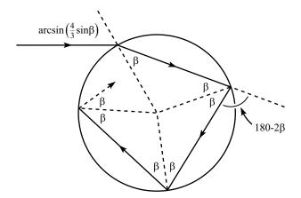
With  $\beta$  defined as in the figure, the light gets deflected clockwise by an angle of  $180-2\beta$  at each reflection point. In addition, it gets deflected clockwise by an angle of  $\arcsin(\frac{4}{3}\sin\beta)-\beta$  at the two refraction points. The total angle of deflection is therefore
