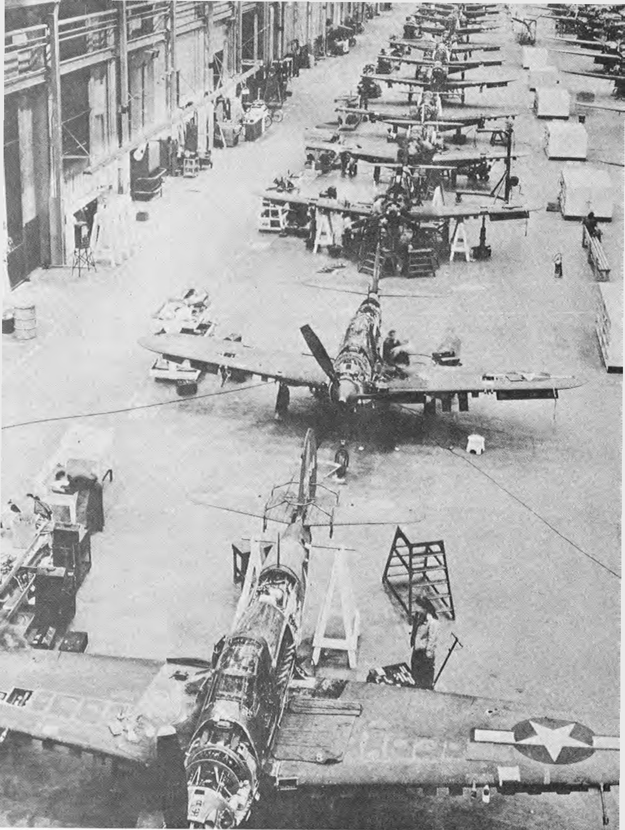
PRODUCTION LINE METHODS IN REPAIR OF P-39'S McCLELLAN FIELD, CALIF.
