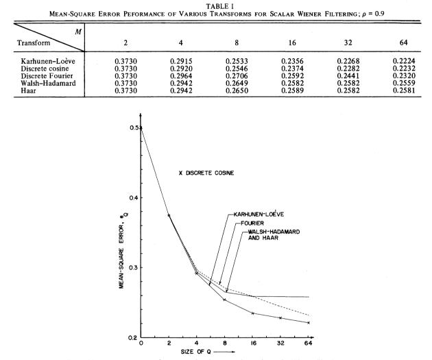
Fig. 4. Mean-square error performance of various transforms for scalar Wiener filtering;  $\rho = 0.9$ .
