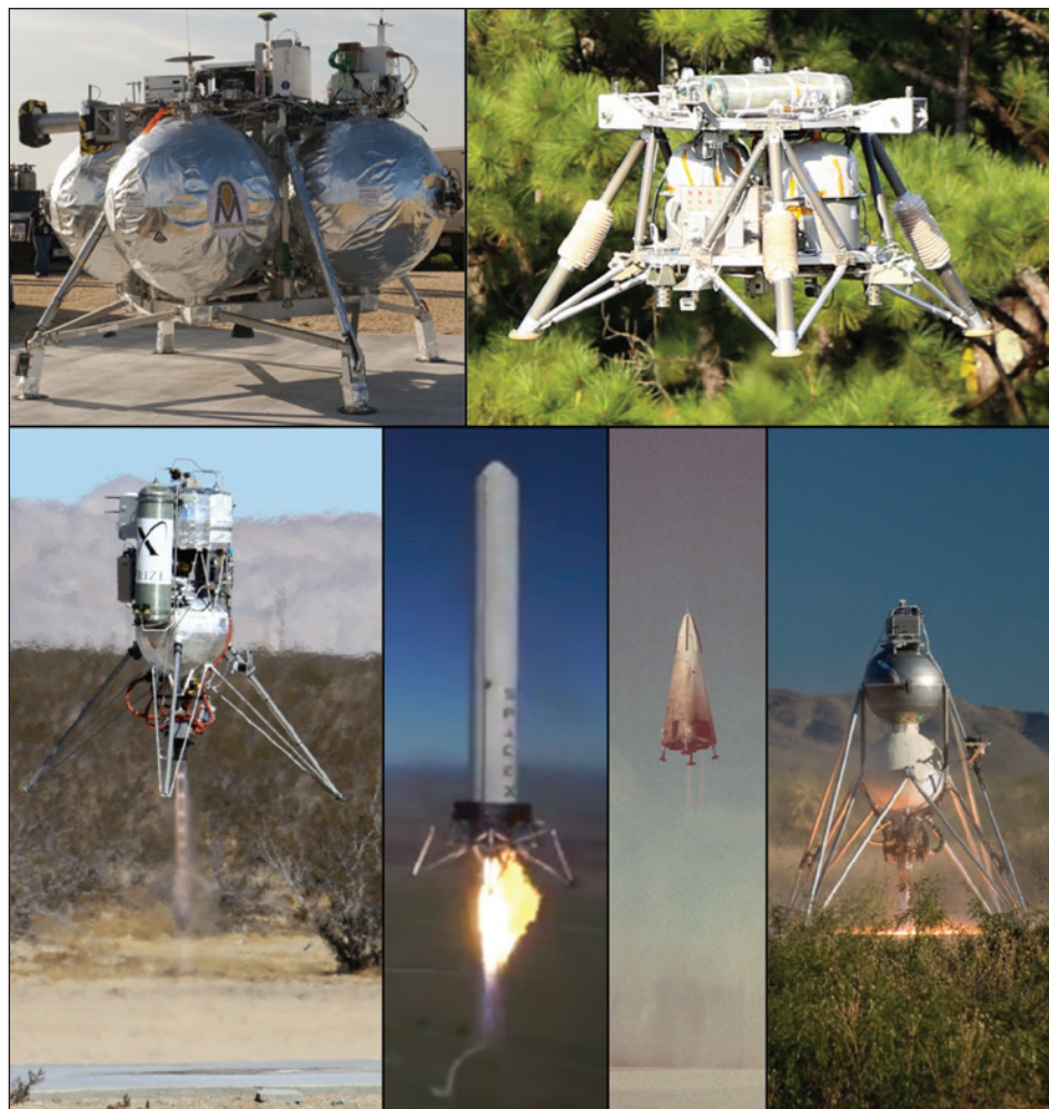
FIGURE 6 Various experimental vertical takeoff and landing testbeds. Clockwise from top left: NASA's Morpheus (left) and Mighty Eagle (right), Masten Aerospace's Xoie , SpaceX's Grasshopper , McDonnell Douglas' DC-X , and Armadillo Aerospace's Mod . Image credits: NASA/Dimitri Gerondidakis ( Morpheus ); NASA/MSFC/Todd Freestone ( Mighty Eagle ); Ian Klufft ( Xoie ); NASA ( DC-X ); Armadillo Aerospace/Matthew C. Ross ( Mod ).
