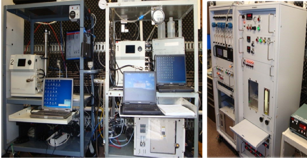
Figure 2: PM and Gaseous Emissions Instrumentation in the TERTEL
