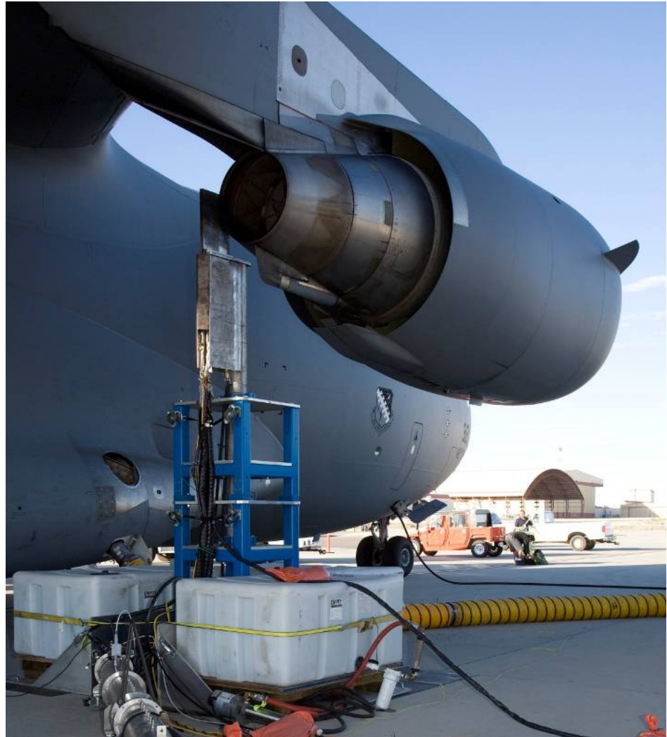
Figure 5: Particle and Gas Probes Installation at F117 Engine Exit Plane
