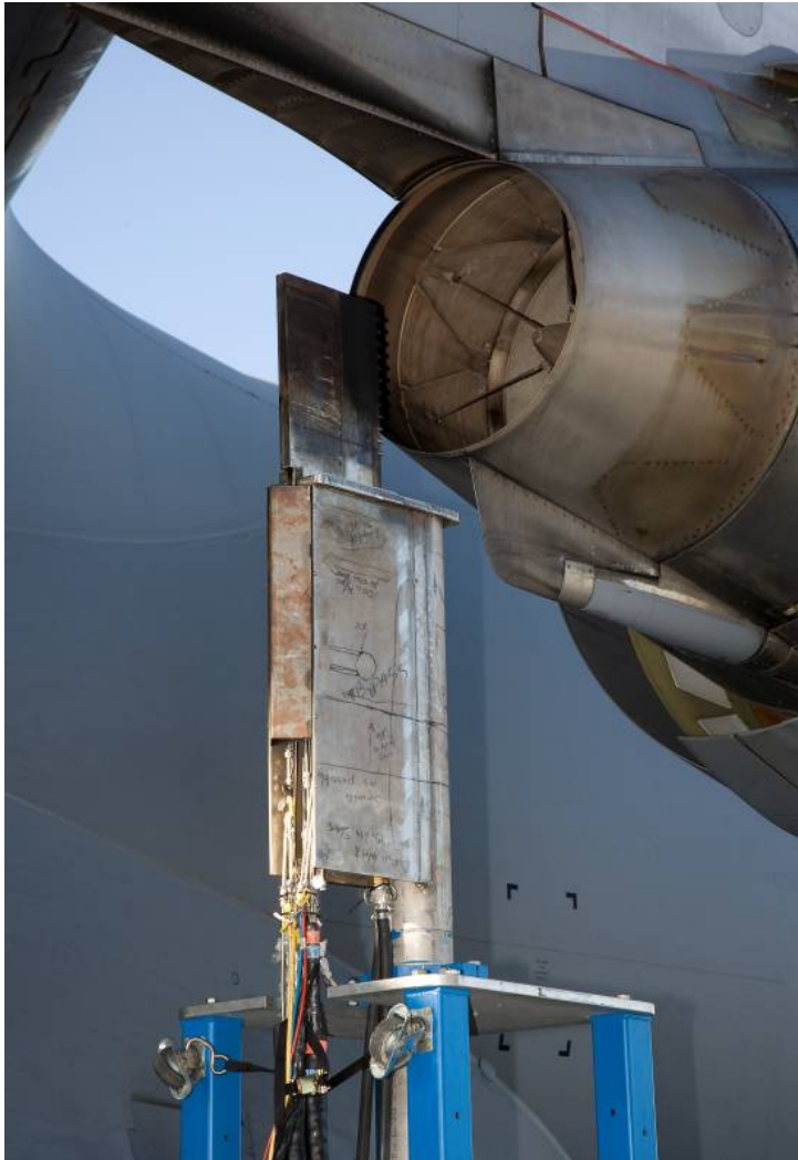
Figure 5: Particle and Gas Probes Installation at F117 Engine Exit Plane
