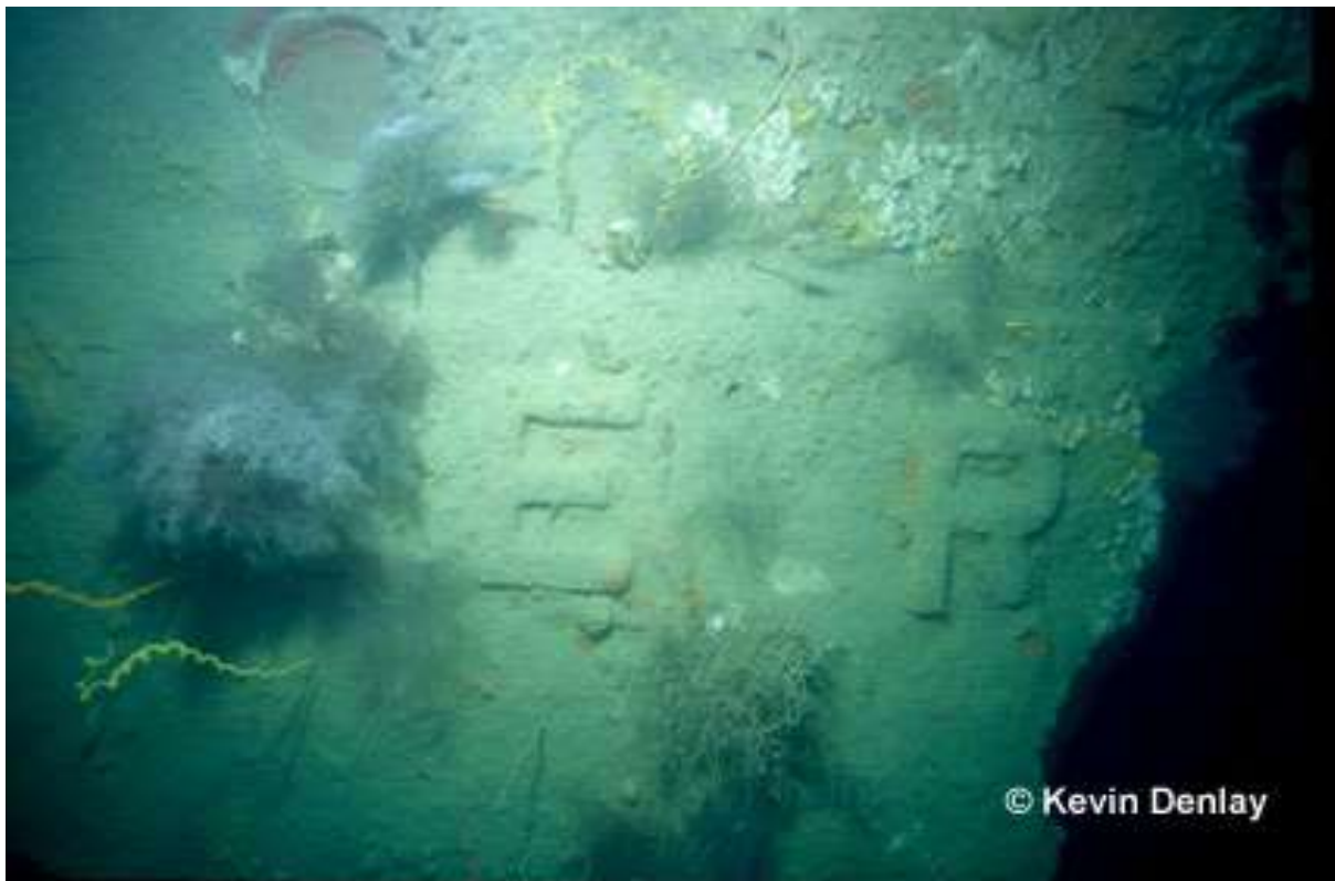
Figure 17: While the letter D is hidden by a small coral bush on left, the letters E and R of De Ruyter's name, as seen in historical photos on her stern, are clearly visible. A large gash or split runs down De Ruyter's port hull just to the right of the letter R.
