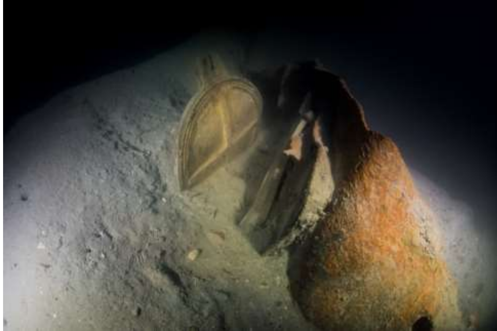
Figure 23: Torn hull plating and scuttle with deadlight at the De Ruyter site. The bronze deadlight with the cross on it is typical of those seen in Dutch cruisers and quite unlike the Admiralty pattern ones on HM and HMA ships.
