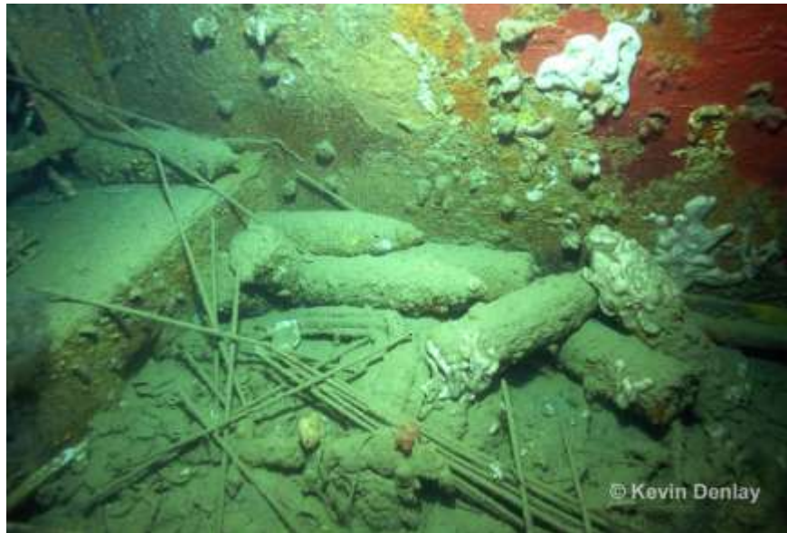
Figure 26: Unused (i.e. 'live' unexploded) 5.9 inch / 150mm projectiles laying against a bulkhead on the Dutch cruiser Hr.Ms. Java . The long thin strips (foreground) are cordite from inside the brass shell casings that would have been loaded with the projectiles.
