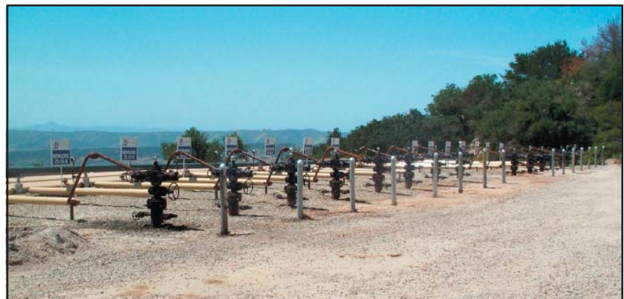
Photo 3. BreitBurn Energy Co. LP selected two drilling pads to directionally drill to exploit resources found on the “Newlove” lease. Cyclic steaming of the Sisquoc diatomite has improved production in the Orcutt oil field. Photo by J. Carnahan.
