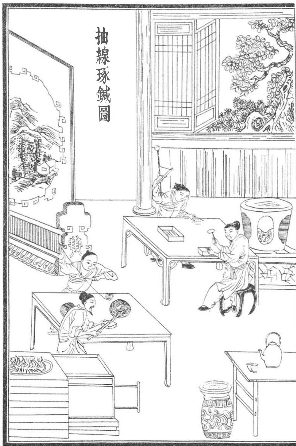
Fig. 332. Steel for magnetised needles: a scene of wire-drawing and needle-making from the Thien Kung Khai Wu (+1637).
