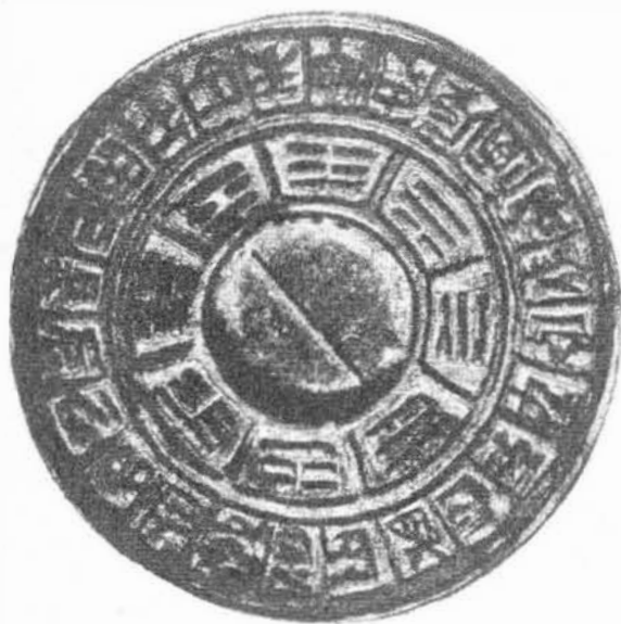
Fig. 333. Mariner's floating-compass of bronze, Ming period, diam. c. 3\frac{1}{2} in. (from Wang Chen-To, 5) South is at 'half-past ten o'clock', and a fiducial line on the bottom of the water-compartment seems to make allowance for a declination slightly west of north. The 24 compass-points in the outer band, the 8 kua in the inner.
