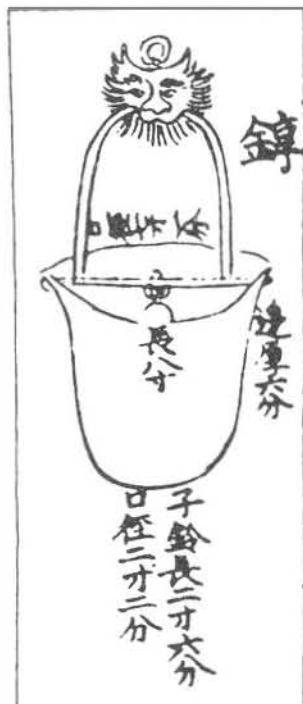
Fig. 317. The chhun , a bronze bell of elliptical section, wide at the mouth and narrowing towards the round base, suspended by a loop usually, as here, in the form of a tiger ( Akhak Kwebōm , ch. 6, p. 24b). Like the ling , it had a tongue, but hung from a crossbar as the chhun was open upwards. Chhun filled with various amounts of water were sometimes used for tuning purposes.
