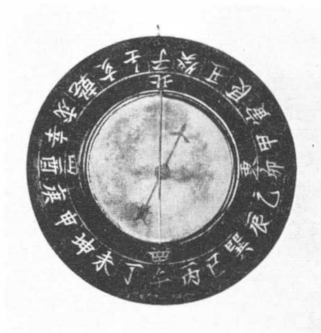
Fig. 337. Mariner's dry-pivoted compass, early Chhing period, diam. c. 3½ in. (Museum of the History of Science, Florence). South is at the bottom. The 24 compass-points in the outer band, the four cardinal directions in the inner.
