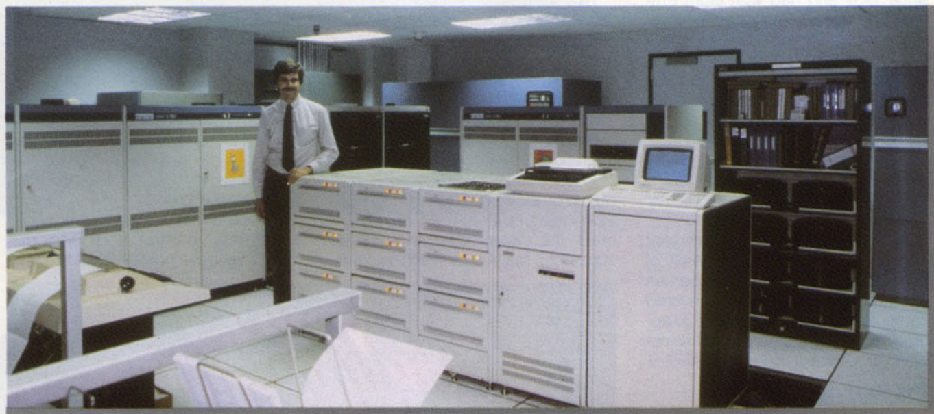
Three VAX 11/780 computers configured as a VAXcluster (with 6 gigabytes of disk storage) form the heart of the Hanna-Barbera computer-assisted animation system.
