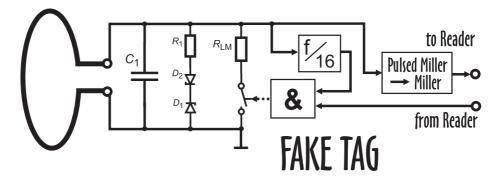
Fig. 4. Operation Principle of the Fake-Tag
