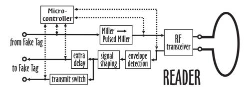
Fig. 3. Operation Principle of the RFID-Reader
