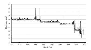
**Fig. 17.** Diameter of hole No. 5G-1 versus depth at different times: 25 January 1998 (thick solid line); 29 December 1999 (dotted line); and 23 January 2006 (thin solid line).
