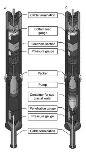
**Fig. 24.** Scheme of thermal drill TBPO-132: (a) without sampler; and (b) with sampler.
