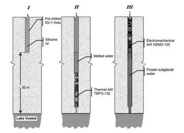
Fig. 23. Scheme of penetration and sampling of Vostok Subglacial Lake.
