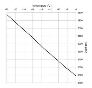
Fig. 15. Temperature profile in the lower part of hole No. 5G.
