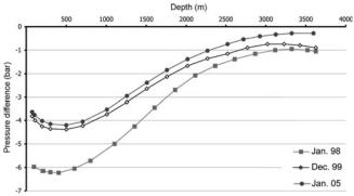
Fig. 18. Pressure difference on the walls of hole No. 5G-1.
