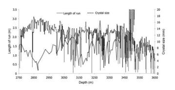
Fig. 19. Length of run and ice crystal size versus depth in hole No. 5G-1.
