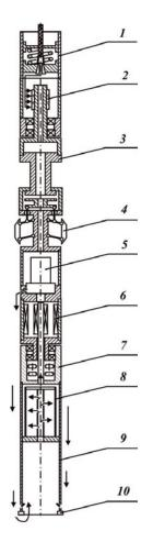
**Fig. 12.** KEMS-112 (KEMS-132) electromechanical drill: 1. cable termination; 2. electric chamber; 3. hammer block; 4. anti-torque system; 5. pump; 6. electric drive motor; 7. reducer; 8. chip chamber including chip filter; 9. core barrel; 10. drill head.
