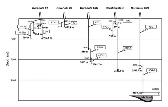
Fig. 6. Schematic of deep holes at Vostok station.
