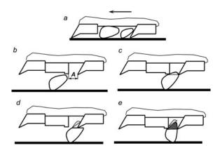
Fig. 21. Scheme of interaction between cutters and oversize pieces of ice.
