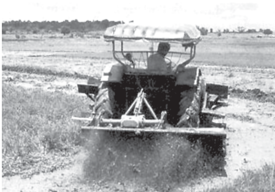
Figure 8. Big four-wheel tractors with rotavating attachment and extension lugwheels for flooded rice fields
