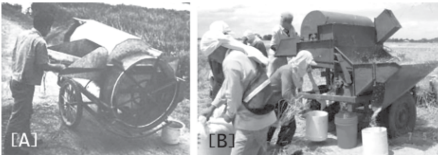
Figure 15. The axial-flow thresher released by IRRI in the early 1970s [A] and a recent commercial model [B]
