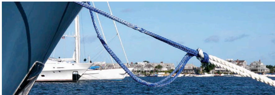
This pendant uses chafe-resistant Dyneema on the boat, coupled with standard stretchy nylon line at the mooring.
