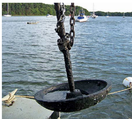
Mushroom anchors can drag if the chain wraps around the shank.
