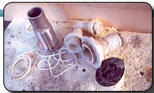
Plastic thru-hulls get brittle and crack, which can sink a boat. They should be replaced with Marelon or bronze.
