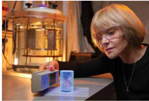
Natalia Zaitseva, an LLNL materials scientist, leads a team of Livermore researchers that has developed the first plastic material capable of efficiently distinguishing neutrons from gamma rays, something not thought possible for the past five decades or so. Photo by Jacqueline McBride
