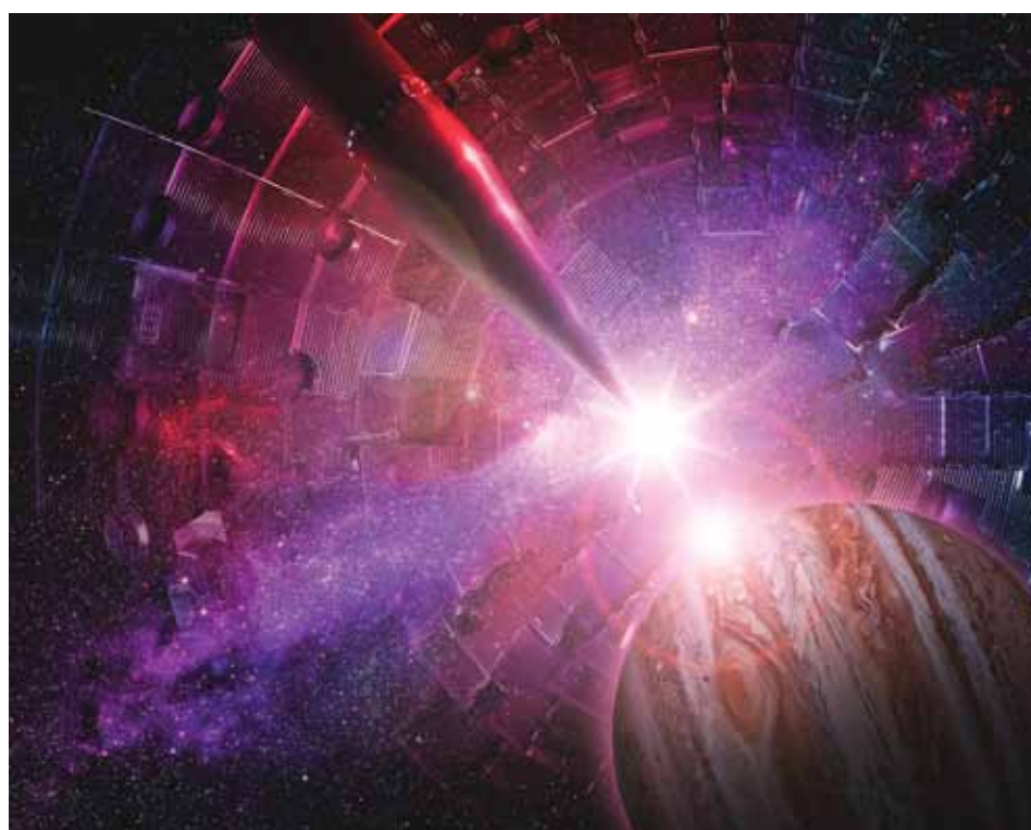
The interior of the target chamber at the National Ignition Facility at Lawrence Livermore National Laboratory. The object entering from the left is the target positioner, on which a millimeter-scale target is mounted. Researchers recently used NIF to study the interior state of giant planets. Image - Damien Jemison/LLNL
