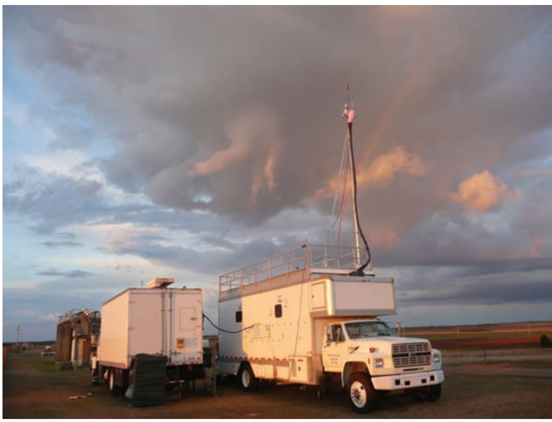
A Sandia-led team built two mobile facilities that are designed to measure greenhouse gases and other species so that they could be traced and identified. The system was deployed recently to the Atmospheric Radiation Measurement (ARM) facility in Oklahoma. (Photo by Hope Michelsen)
