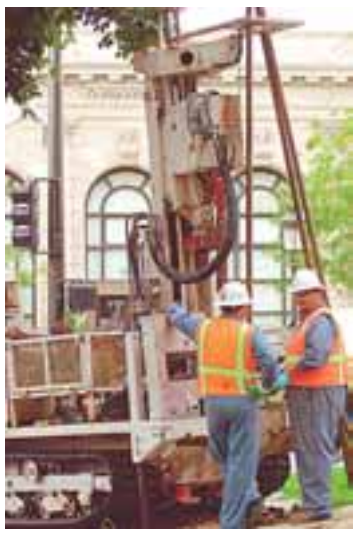
Photo - Doug Jorgensen Workers spent the last few days testing soil at a former gas station site at the corner of First St. and Livermore Avenue.
