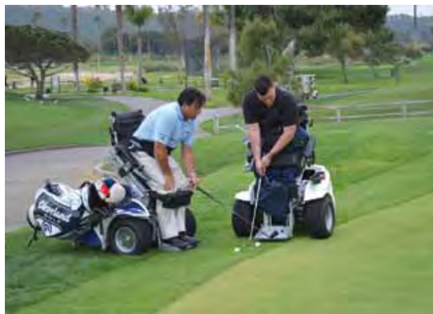
Paramobile is a multi-terrain vehicle that allows disabled persons to stand.
