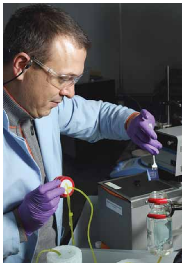
Sandia National Laboratories researcher Vitalie Stavila inserts a substrate patterned with electrodes into a temperature-controlled liquid-phase reactor for depositing MOF thin films. Sandia's research team plans to combine MOFs with dye-sensitized solar cells, a technique it believes will lead to advancements in photovoltaic technology. (Photo by Dino Vourmas)
