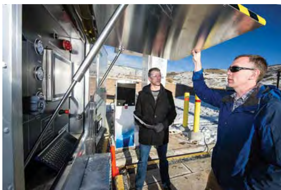
Sandia National Laboratories mechanical engineer Terry Johnson, left, the project leader for the Hydrogen Station Equipment Performance (HyStEP) device, and National Renewable Energy Laboratory researcher Chris Ainscough prepare HyStEP for testing at NREL's Energy Systems Integration Lab. HyStEP will accelerate hydrogen refueling station commissioning. (Photo by Dennis Schroeder/NREL)
