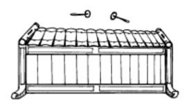
Gendèr, a metallophone with bronze keys suspended by cords in a wooden frame, over tube resonators. It is played with two tabuh of the disc type (i.e. padded disc which is attached to the end of a stick). There are two kind of gendèr: gendèr barung and gendèr panerus. The gendèr barung can have as few as twelve or as many as fourteen keys, encompassing more than two octaves. A sléndro gamelan has one gendèr. The pitches are:
