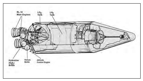
Figure 2–26. Pratt & Whitney RL10 Engine used on the Centaur Upper Stage. (Pratt & Whitney)
