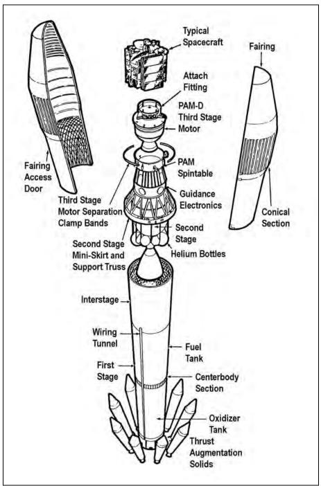
Figure 2–13. Delta II Components. (The Boeing Company)
