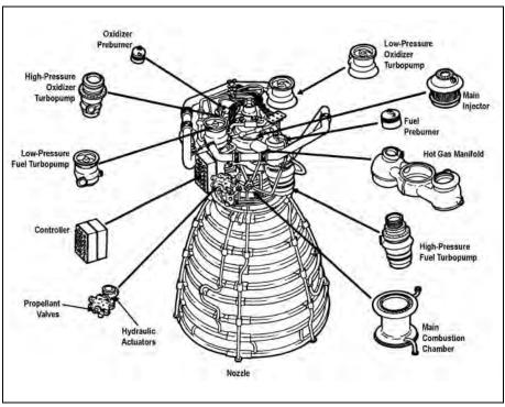
Figure 2–24. Space Shuttle Main Engine Components. (Rocketdyne)
