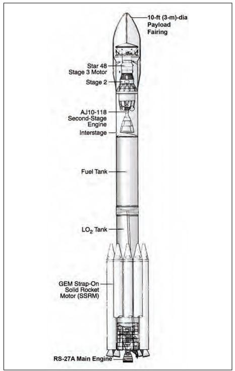
Figure 2–14. Delta II 7925. (The Boeing Company)
