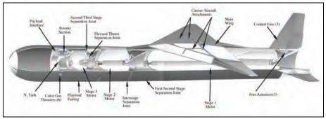
Figure 2–18. Pegasus Vehicle. (Orbital Sciences Corp.)
