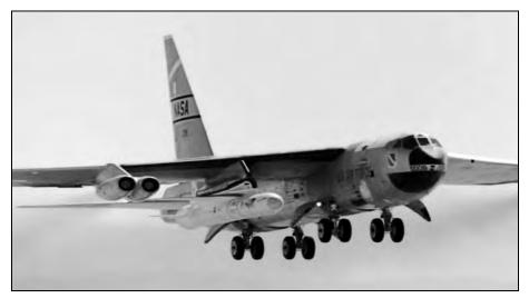
Figure 2–17. Pegasus Mounted Under B-52 Wing. (NASA-DFRC Photo No. EC91-348-3)
