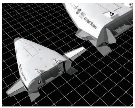
Figure 2–32. Artist's concept showing the relative size of the X-33 (left) and the proposed operational VentureStar. The VentureStar was to be twice the size of the half-scale X-33. (NASA-DFRC Photo No. ED97-43938-1)
