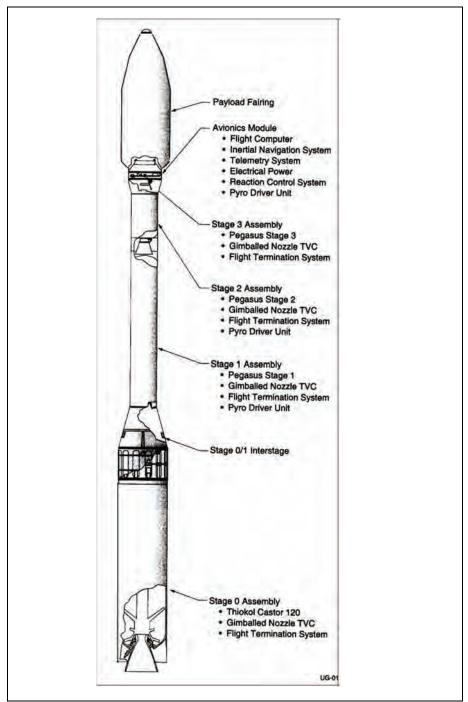
Figure 2–20. Taurus Launch Vehicle Configuration. (Orbital Sciences Corp.)
