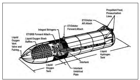
Figure 2-22. Drawing of Space Shuttle External Tank. (NASA)
