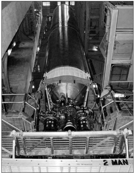
Figure 2–21. The first stage of the Titan IV ELV that sent NASA's Cassini Spacecraft to Saturn and its moon. Titan is Llowered into a high bay in the Vertical Integration Building at Cape Canaveral Air Station to begin stacking operations, April 14, 1997. (NASA Photo No. KSC-97PC-640)
