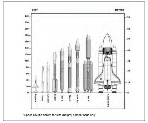
Figure 2–1. NASA's Fleet of Launch Vehicles (1989–1998). Not Pictured: the Scout and the Conestoga. The Scout stood 75 feet (23 meters) tall, placing it between the Pegasus and Taurus. The Conestoga stood 50 feet (14 meters), making it about the same height as the standard Pegasus.
