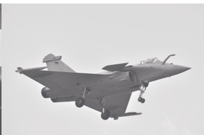
Safran's contribution to the Rafale fighter (non-exhaustive): M88-2 engines (Safran Aircraft Engines). Wiring (Safran Electrical & Power). Inertial navigation system (Safran Electronics & Defense). Landing gear (Safran Landing Systems). Wheels and carbon brakes (Safran Landing Systems). Ejection seats (SEM MB).
