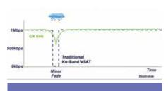
Adaptive Coding and Modulation (fwd link) and A-TDMA (rtn link) used in GX network enables the system to assign more power or to gracefully slow throughput to avoid link loss
