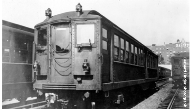
A Gibbs car after modification for Multiple Unit Door Control (MUDC) in 1936.
