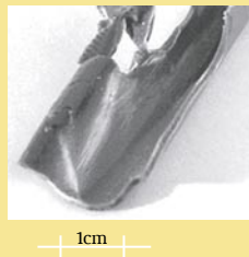
Figure 5: Fragment of the deformed fuel rod (reconstruction)
