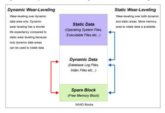
In the past, the more tolerant, earlier generations of NAND flash were managed by Dynamic Wear-Leveling, a simpler algorithm that utilizes only the dynamic area for wear-leveling. But due to increased issues of reliability with newer generation NAND flash, a more advanced and complex method, Static Wear-Leveling, which utilizes both static and dynamic areas for wear-leveling, is becoming more prominent in future SSD designs.
