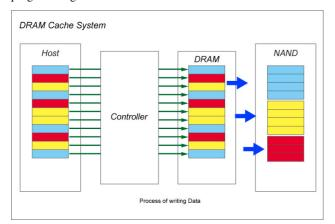
By effectively utilizing cache to temporarily store fragmented data, which is organized into larger blocks of data, the SSD can avoid inefficient programming and gain an improvement of NAND flash longevity.
