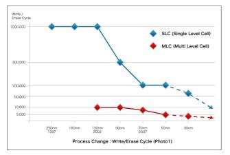
In order to deal with these issues, the SSD device must have the capability to monitor and obtain accurate Program/Erase Cycle Count and Read Count internally based on the user's actual usage.
