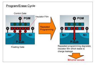
Design-rule shrink affects the insulator film, reducing tolerance due to repeated programming. For this reason, current 56nm MLC NAND flash can only tolerate 5,000 program cycles where in comparison older 90nm MLC NAND flash could tolerate 10,000 program cycles.
