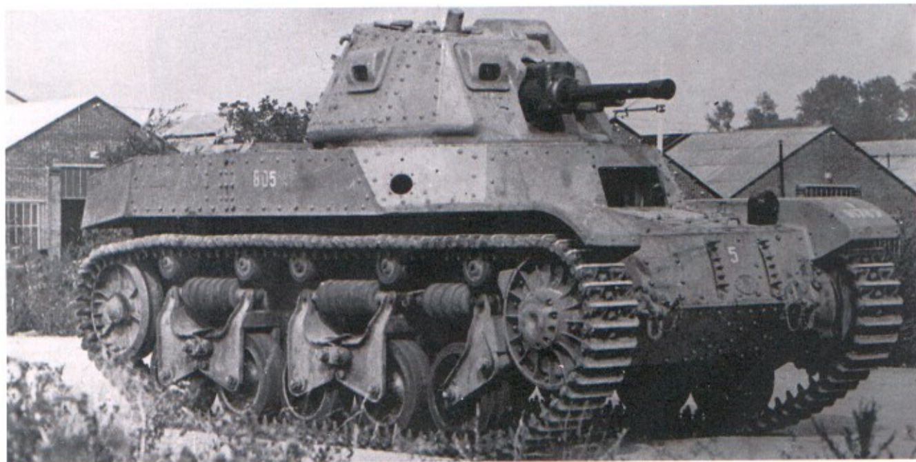
Above: The Renault AMC 35 light tank (also known as the ACGI) mounted a 47mm gun and weighed 14.5 tons. (TM)
