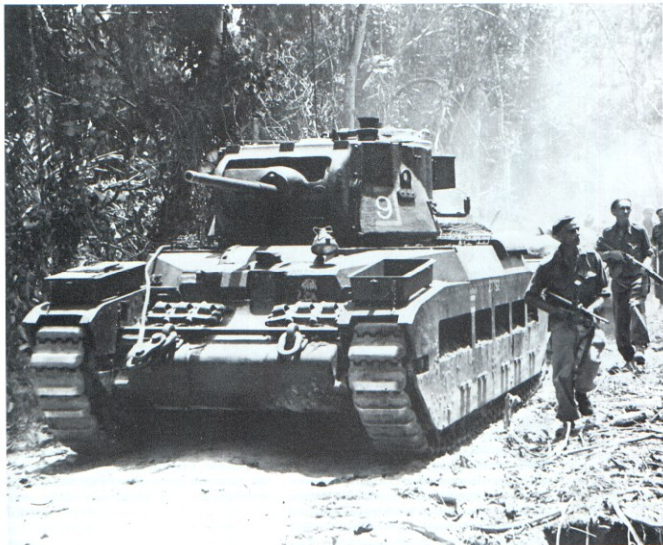
Above: Matilda II of 2nd Battalion, 4th Australian Armoured Regiment on the Buin Road, Bougainville, New Guinea, April 1945. Note the spotlight mounted next to the driver's hatch. (TM)
