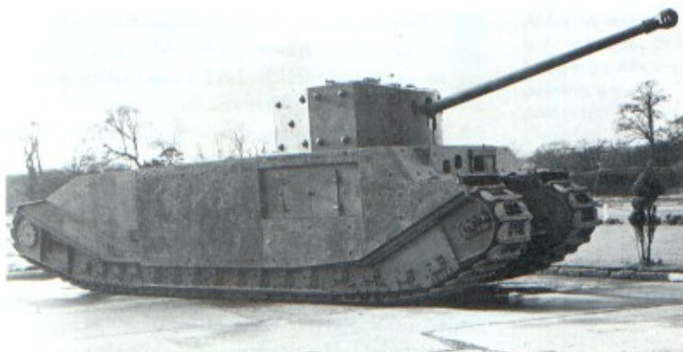
Top: Tortoise, the A39 heavy assault tank, only six were built in pilot form. (TM)
