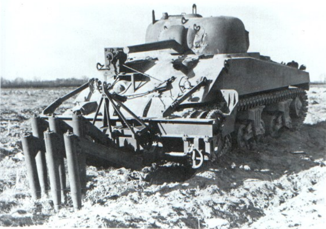
Left: The Mine Exploder T8, also known as 'Johnnie Walker' a six steel plunger exploder unit on a pivoted frame. It proved impossible to steer and was abandoned. (TM)
