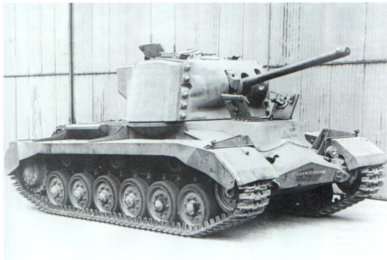
Above: The 27ton A38 Valiant was designed as an improved version of Valentine, but was 10 tons heavier. Underpowered it never entered production, being cancelled in 1945. The surviving A38 is in the Tank Museum, Bovington. (TM)
