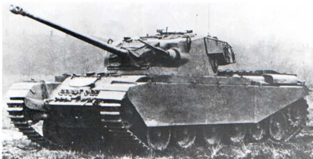
Right: The A41 Centurion Mk I was the first of a highly successful line of medium gun tanks which continued for over 25 years. Armament is a 17 pounder gun and a 20mm Polsten cannon (only fitted to pilot models, later a co-ax BESA MG was fitted). (TM)
