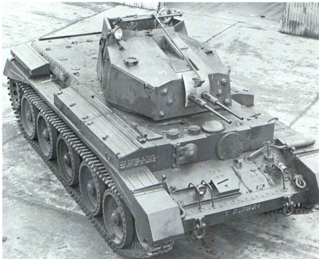
Below: A Centaur AA Mk II, mounted 20mm Polsten cannons on a Centaur III or IV chassis. A similar mounting was tried on the Crusader, but with twin Oerlikon cannons. (TM)
