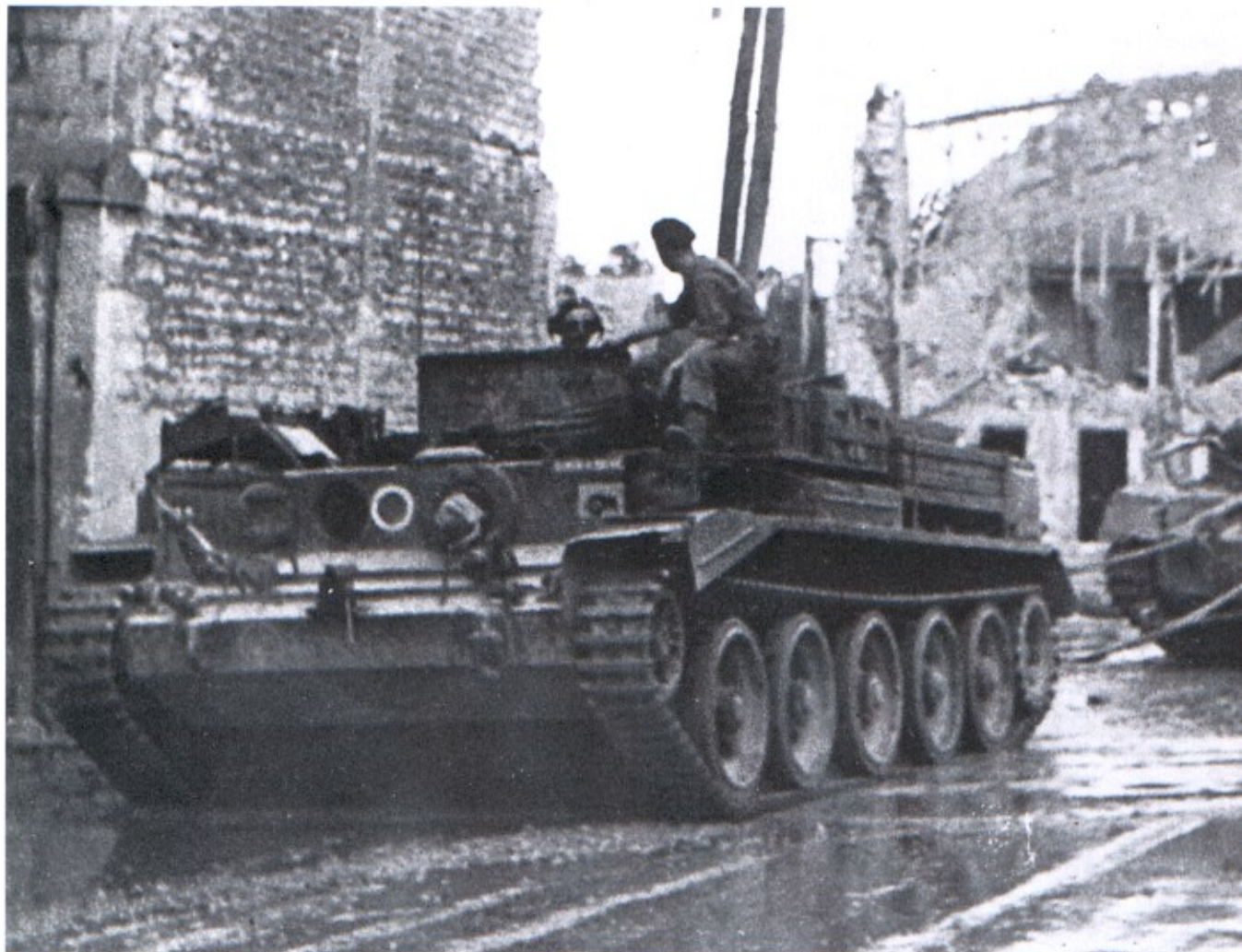
Above: A Cromwell ARV from 11th Armoured Division, towing a captured late model PzKpfw IV. Note the spaced armour around its turret to protect from Bazooka-type projectiles. (TM)
