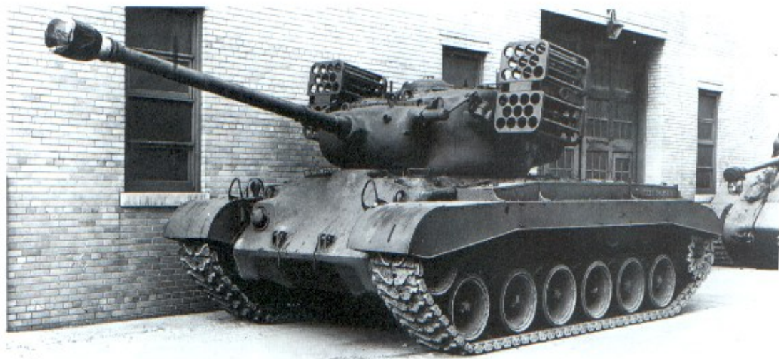
Left: Pershing with the T99 multiple rocket launcher. This was tested in 1945 and could fire forty-four 4.5in rockets from the jettisonable launcher frame. (TM)
