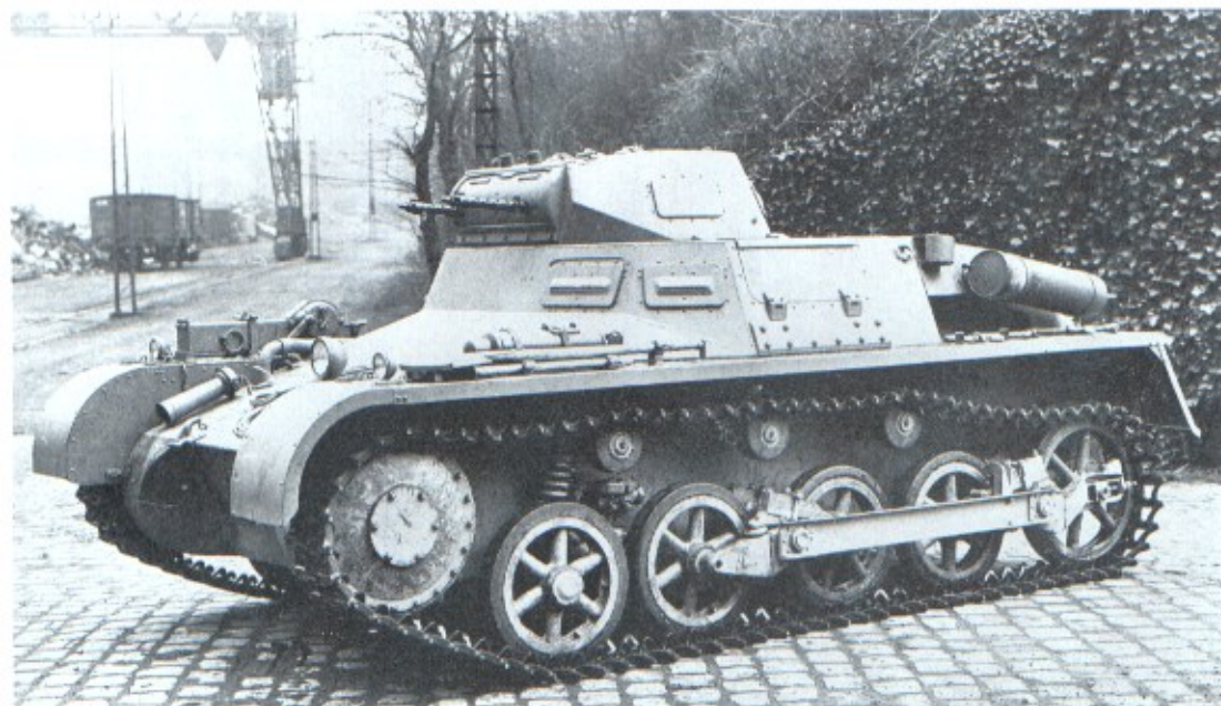
Left: A PzKpfw I Ausf A. Over 2 tons lighter than the Ausf B, its suspension comprised a sprocket, four road wheels and a slightly larger fifth road wheel which acted as the idler, plus three top rollers. The photograph is of a brand new diesel engine Ausf A taken at the Henschel works, Kassel, Germany. (TM)
