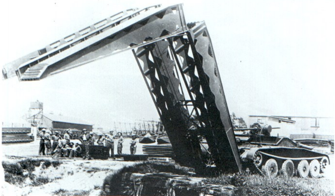
Below: A Covenanter bridgelayer launching its 30ft folding bridge. They were used mainly for training and development work, but a few were used by the Australians in Burma, 1942. (TM)
