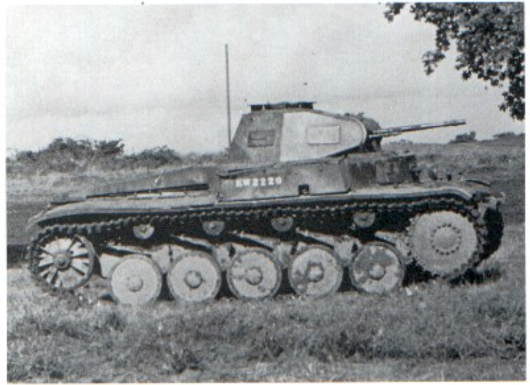
Above and left: PzK pfw II Ausf A, B and C , all had five independently sprung, larger diameter road wheels instead of the earlier six small road wheels. Armament was a 20mm cannon with a co-ax MG 34. (TM)
