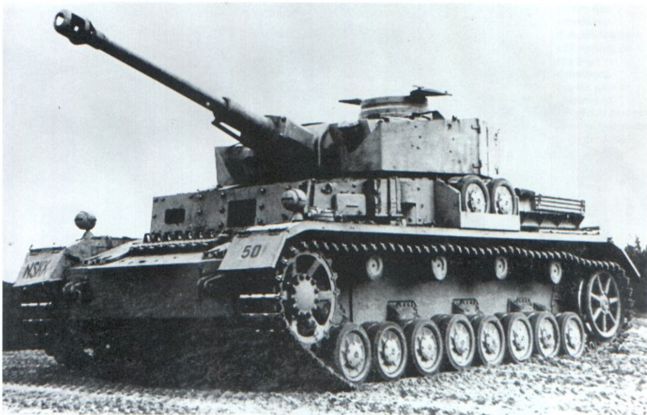
Above: This up-gunned PzKpfw IV Ausf D is fitted with a 75mm KwK L/48 gun and also additional spaced armour around the sides of the turret. (TM)
