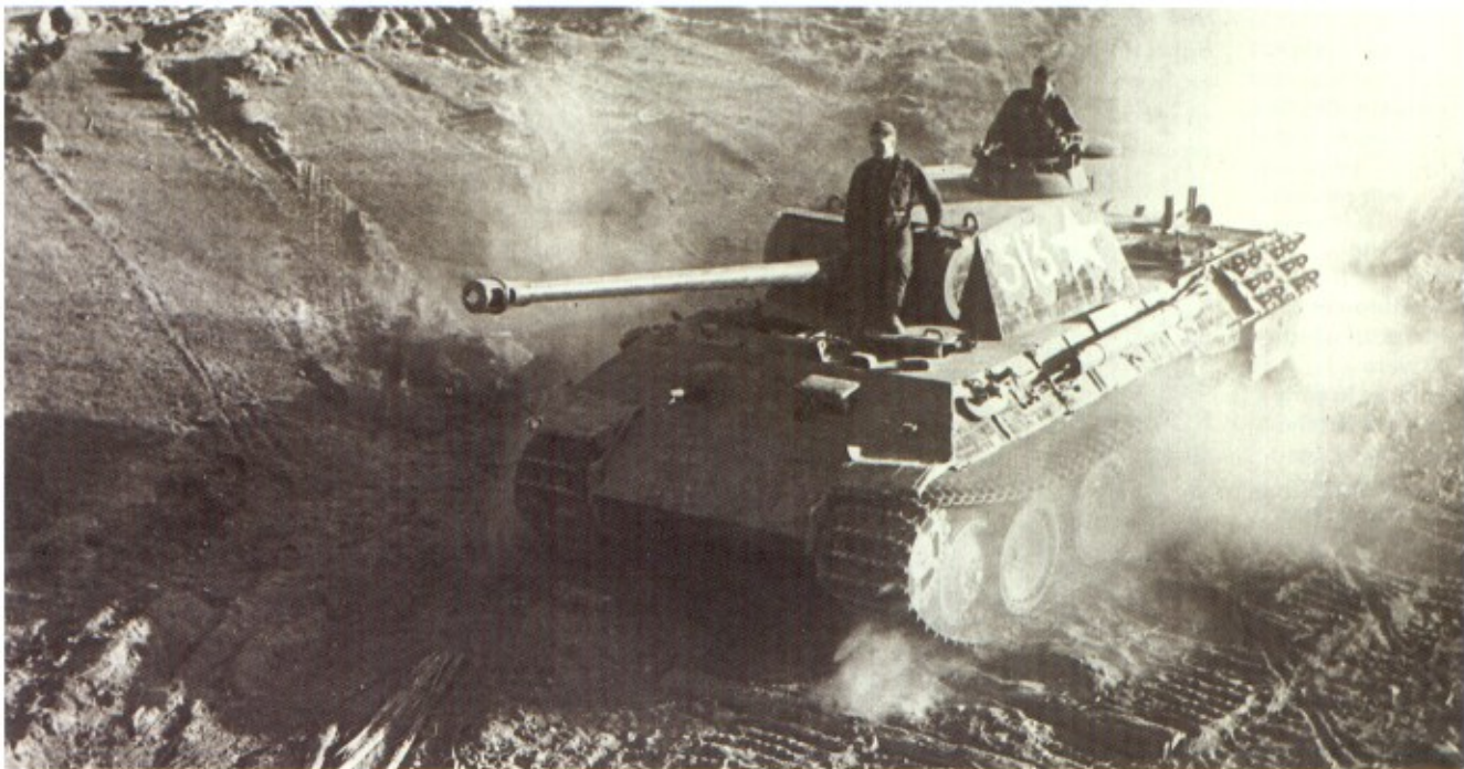
Above: This Panther, PzKpfw V Ausf A has been captured undamaged by the Red Army and is being driven at speed (possibly on test) - its top speed was just under 29mph. (TM)
