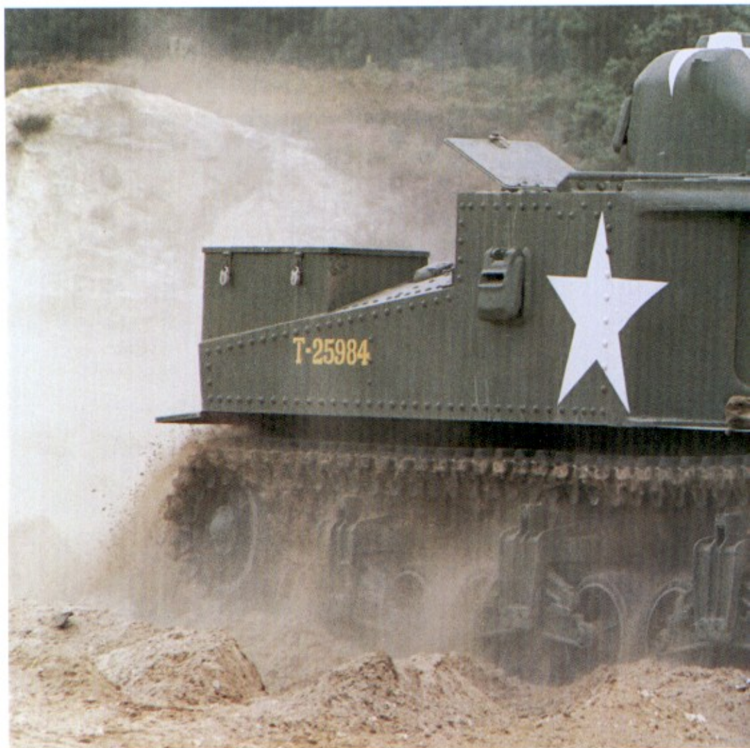
Above: M3 General Grant in desert camouflage. Note the canvas dust cover over the sponson-mounted gun's mantlet. (TM)
