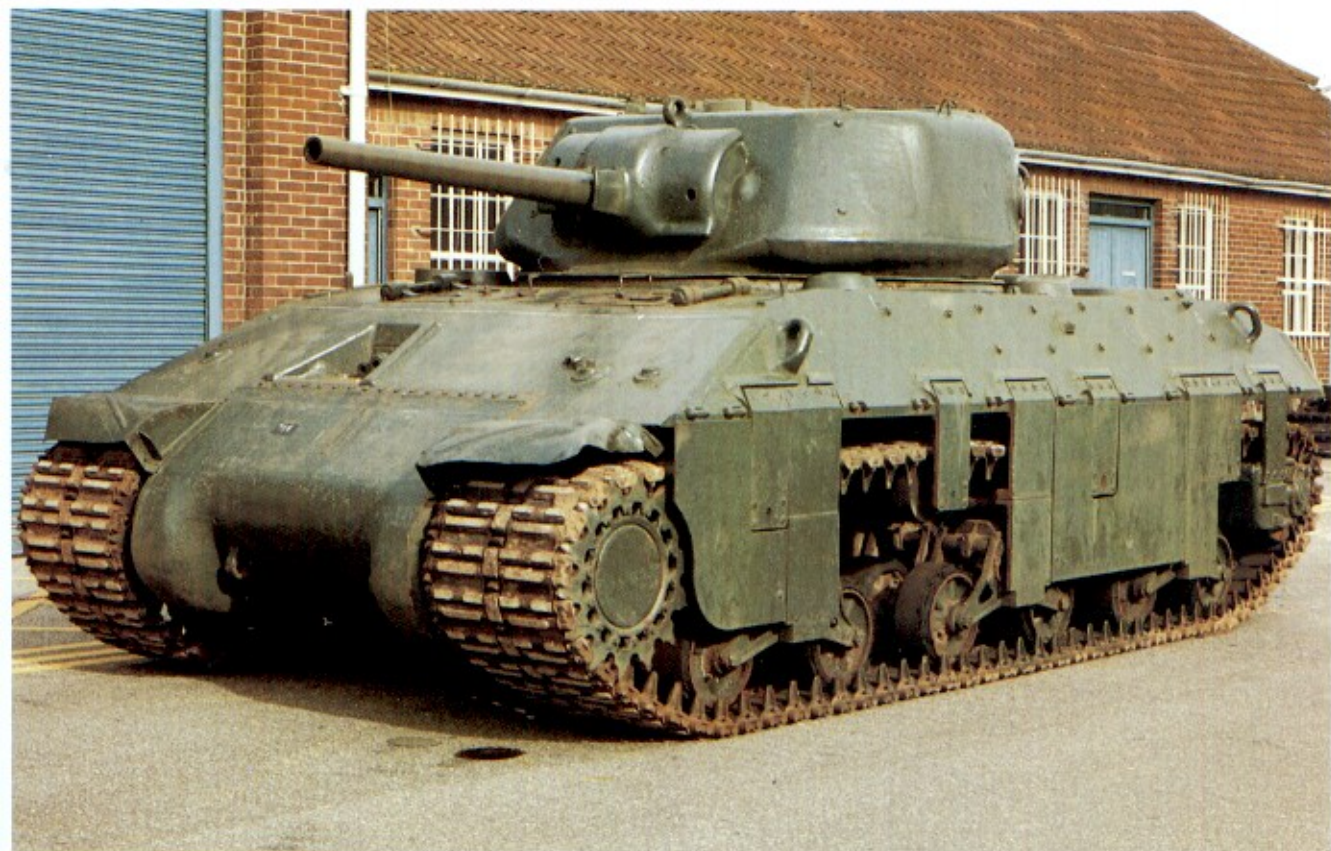
Above: Only two pilot models of the 47-ton Assault Tank T 14 were ever built. In August 1943, one was sent to Britain and the other being tested in the United States. The project was cancelled four months later, but the T14 sent to Britain has been preserved at the Tank Museum. (TM)
