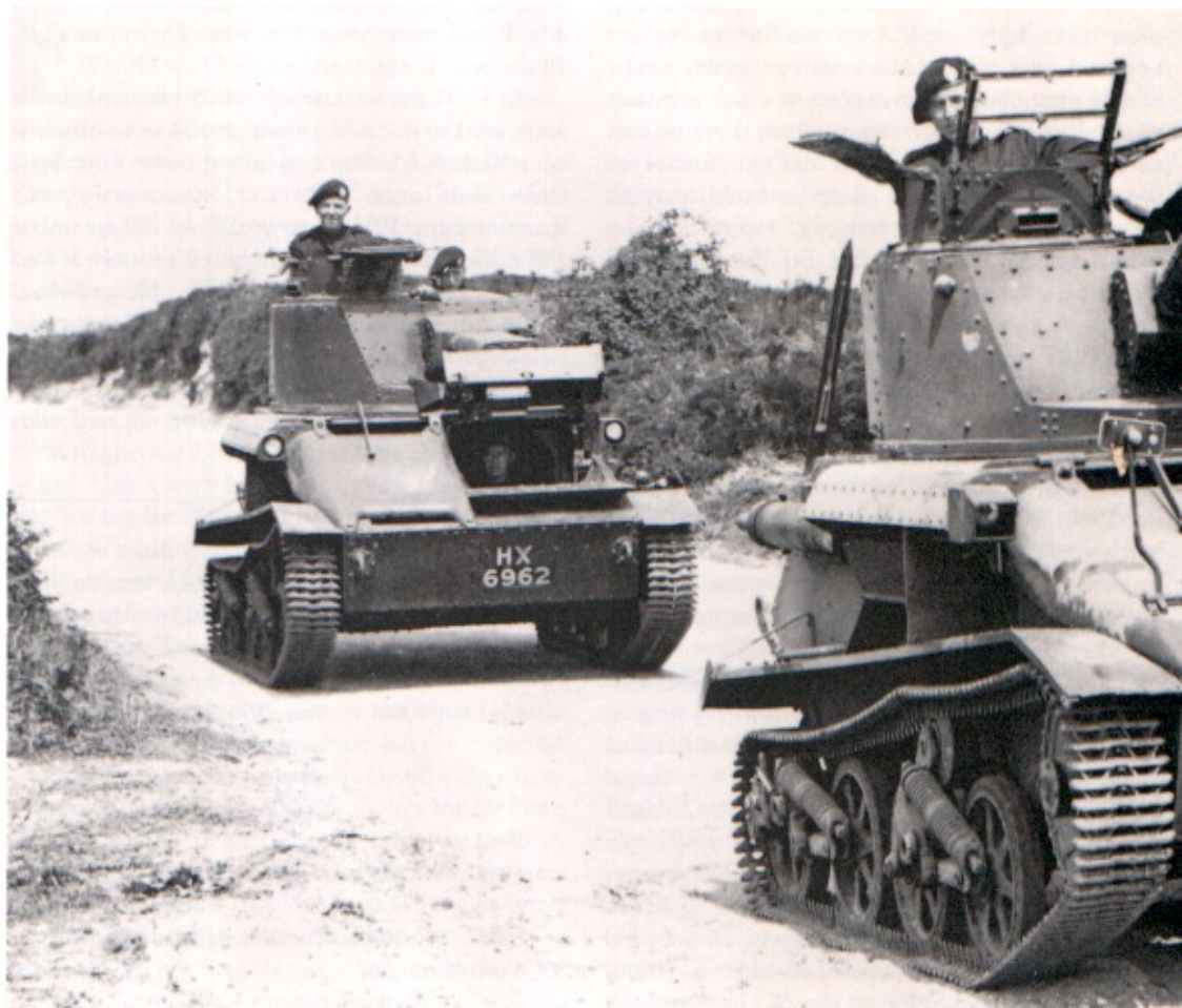
Above: A Light Mk IIB (India pattern) on trials in India, 1935. These little tanks did extremely well, especially over the rough terrain of the North West Frontier. Note the square-shaped non-rotating cupola on top of the turret. (TM)
