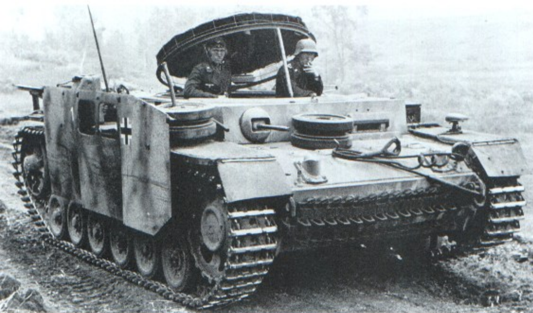
Left: This old PzKpfw III has been converted to a Munitionspanzer (ammunition carrier) by removing the turret. (TM)
