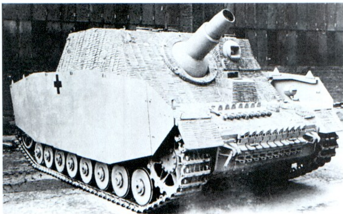
Left: Sturmpanzer IV Brummbär (Grizzly Bear), 150mm assault howitzer on a PzKpfw IV chassis. Just under 300 were produced and rushed to the Eastern front to take part in the Kursk offensive in 1943. (TM)
