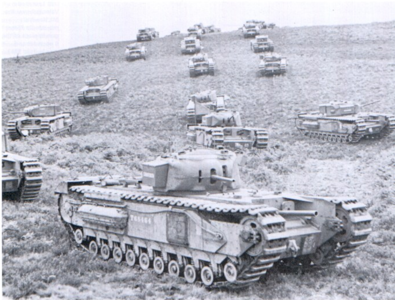
Above: Early Churchills on a training exercise in the New Forest, England - leading is a Mk I with a nose mounted 3-inch howitzer, others are Mk IIs with the howitzer removed and replaced by a BESA machine gun. (TM)
