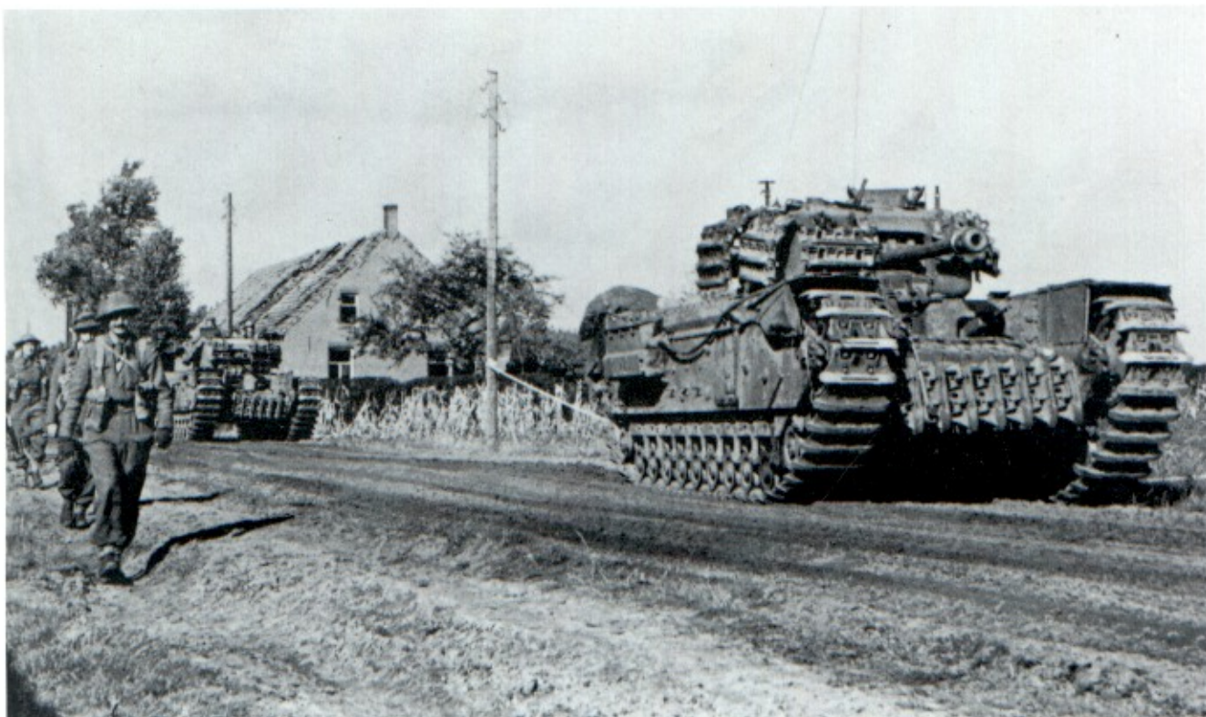
Above: Churchill Mk VI of 4th Battalion Grenadier Guards and accompanying infantry of 1st Battalion Suffolks advance through a Dutch village, 1944. Note the extra armoured protection by adding trackplates to the front glacis and turret. (TM)
