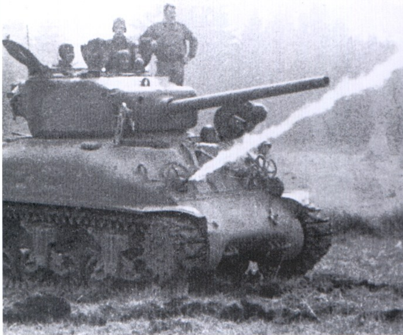
Above: A Sherman M4A1 (76mm gun) mounting an M3-4-3 flamegun in place of the hull machine gun. It had a range of approximately 60 yards. (TM)
