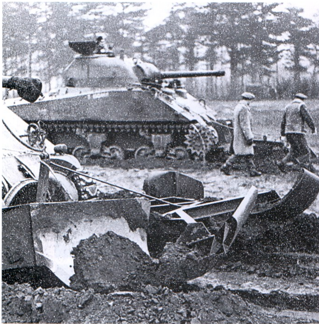
Above: The British-invented Bullshorn Plough had one ploughshare fitted ahead of each track. They were used by the 79th Armoured Division on the Normandy beaches, 1944. The photograph is of the equipment on trials in a snow storm. (T.M.)
