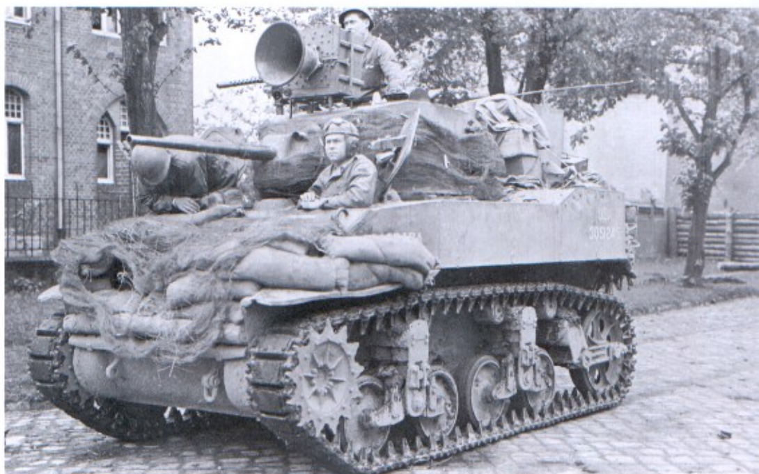
Above: An M3A1 light tank being towed to a field repair base, during training in Britain, prior to D-Day. This version had an all-welded hull and turret. (TM)
