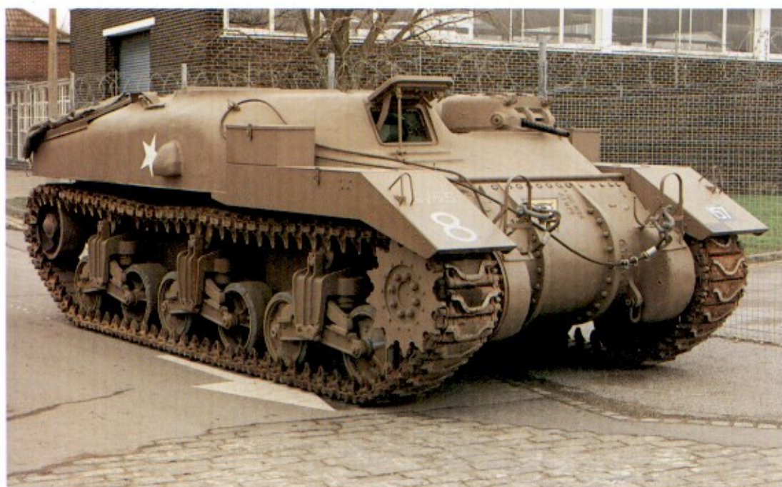
Above: Sherman M32 Tank Recovery Vehicle, was equipped with a jib and a powerful 60,000lb winch. It also mounted an 81mm mortar, so that a smoke screen could be created as cover for operations (not fitted on this vehicle). (TM)
