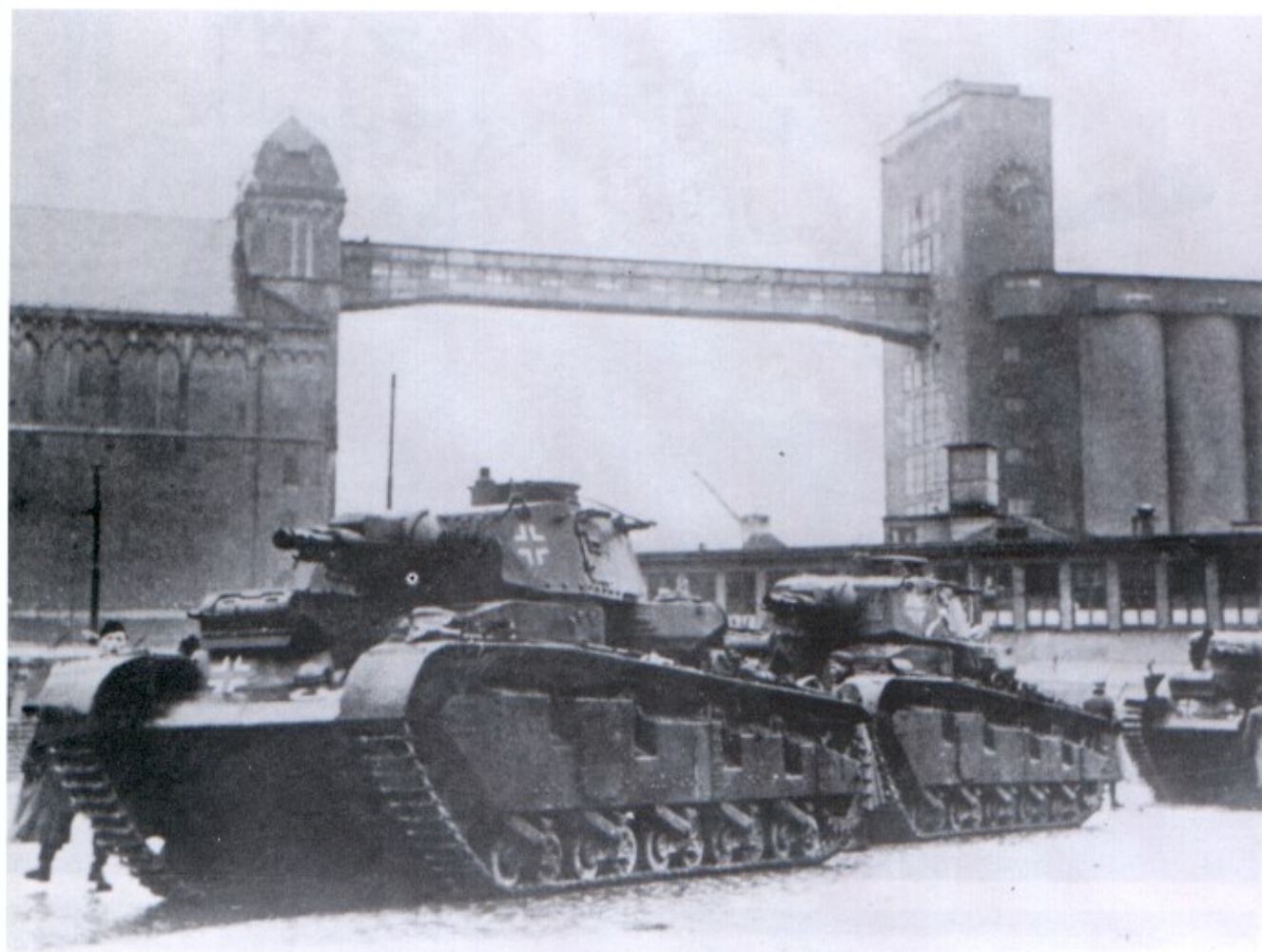
Above: The Neubaufahrzeug medium tank (sometimes known as PzKpfw VI) was ordered from Rheinmetall in 1933 and was to be the first German multi-turreted medium tank. Two prototypes and three experimental vehicles were produced. The latter were sent to Norway in April 1940, where they were used in action, one being destroyed. Photographed in Oslo, 1940. (TM)
