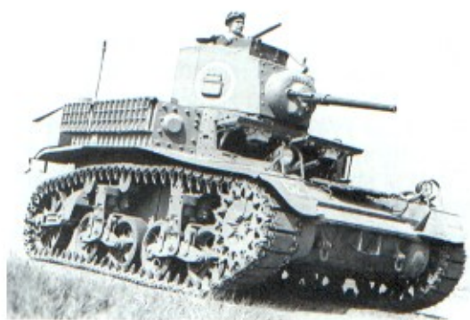
Left: The M3 in Canadian service, where it was known as the Stuart I. Note the side machine gun sponsons have been blanked off. (TM)
