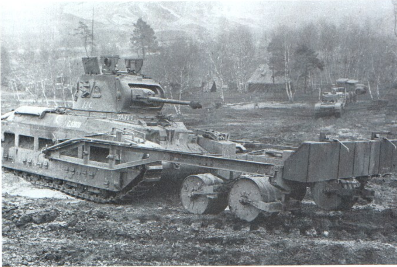
Above: Matilda II, pushing Heavy Carrot mine clearing device – a 600lb demolition charge carried in front of AMRA and detonated remotely from the tank. Photographed at the Obstacle Assault Centre. (TM)
