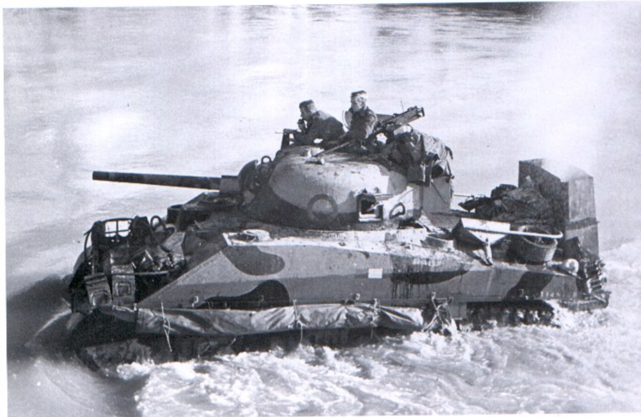
Above: Fording a river in Italy, this Sherman M4A2 (Sherman III) has been fitted with wading trunking over the engine air intake, to keep it clear of water. (TM)
