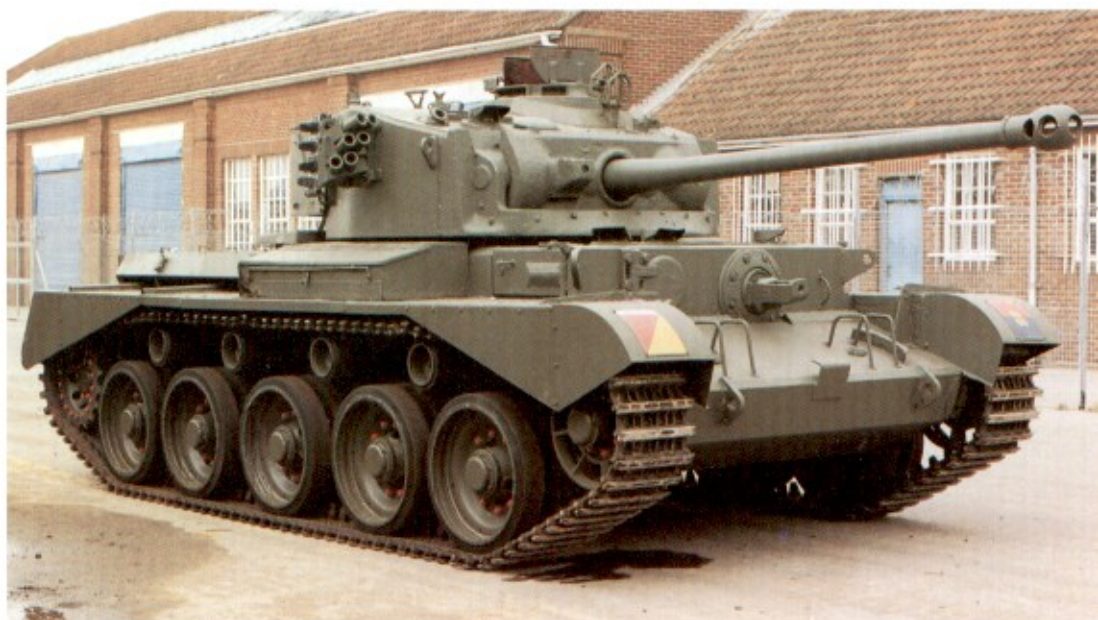
Right: Best of the British Cruiser Tanks of World War Two, the A34 Comet. It continued in service after the war until replaced by Centurion in 1960. The 76.2mm gun had a performance comparable with that of the heavier German tanks. (TM)
