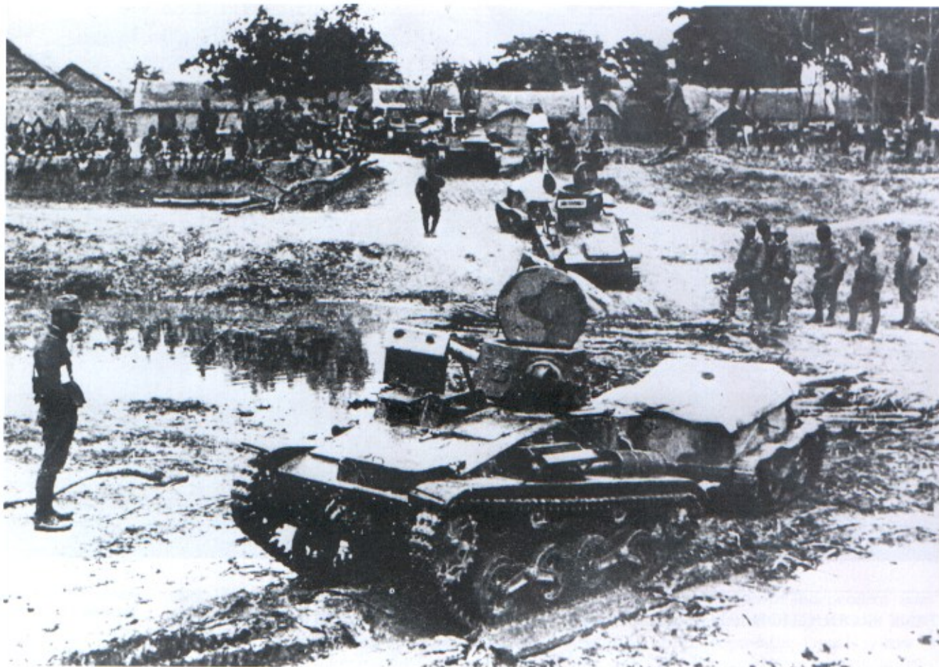
Above: These tankettes, fording a stream in China, are towing light tracked trailers. A diesel version of the Type-94 TK was built but only as a prototype. (TM)
