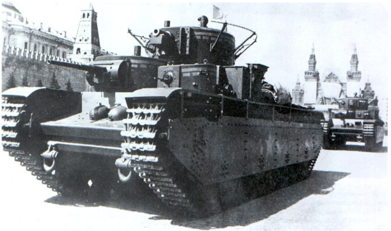
Above: The T-35 heavy tank weighed 45 tons, the main turret mounting a 76.2mm howitzer, while two of the four sub-turrets had 37mm guns and two machine guns. Shown is the commander's version in a parade on Red Square, Moscow. (TM)
