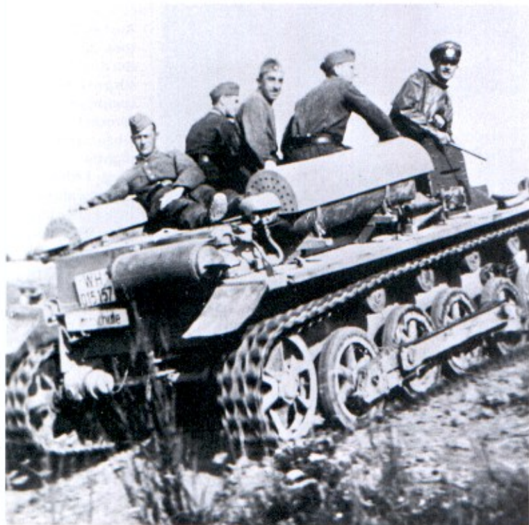
Above: Some driver training vehicles were modified to run on gas – note the gas cylinders on the sides of this PzKpfw I Ausf B ohne Aufbau . (TM)
