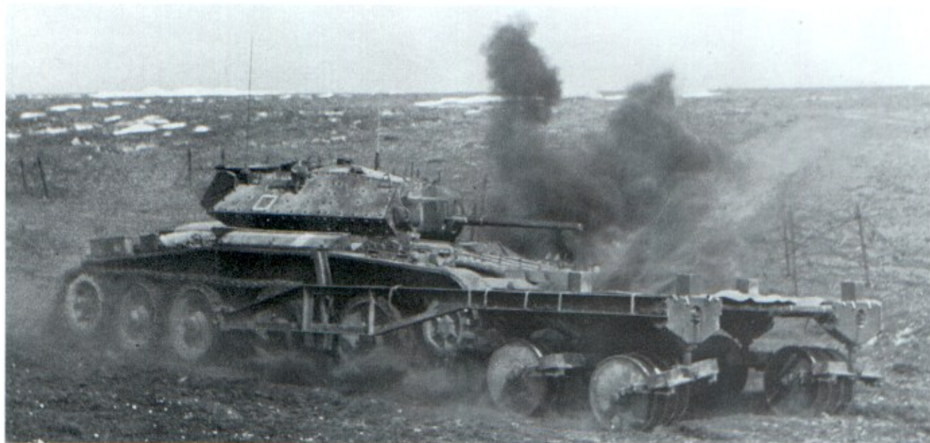
Above: The A13 Mk III (Cruiser Mk V) Covenanter, fitted with an Anti-Mine Roller Attachment (AMRA) on test, 1942. (TM)
