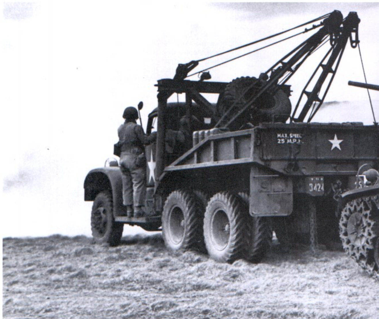
Above: An M3A1 light tank being towed to a field repair base, during training in Britain, prior to D-Day. This version had an all-welded hull and turret. (TM)
