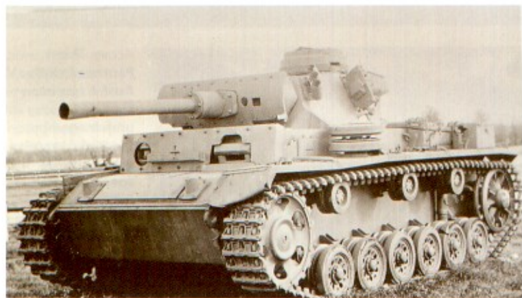
Right: The PzKpfw III Artillerie-Panzerbeobachtungswagen (armoured artillery OP) used a gun tank chassis without turret armament – the dummy gun and centrally-placed machine gun were mounted on a thicker mantlet, the lower MG was also removed. (TM)
