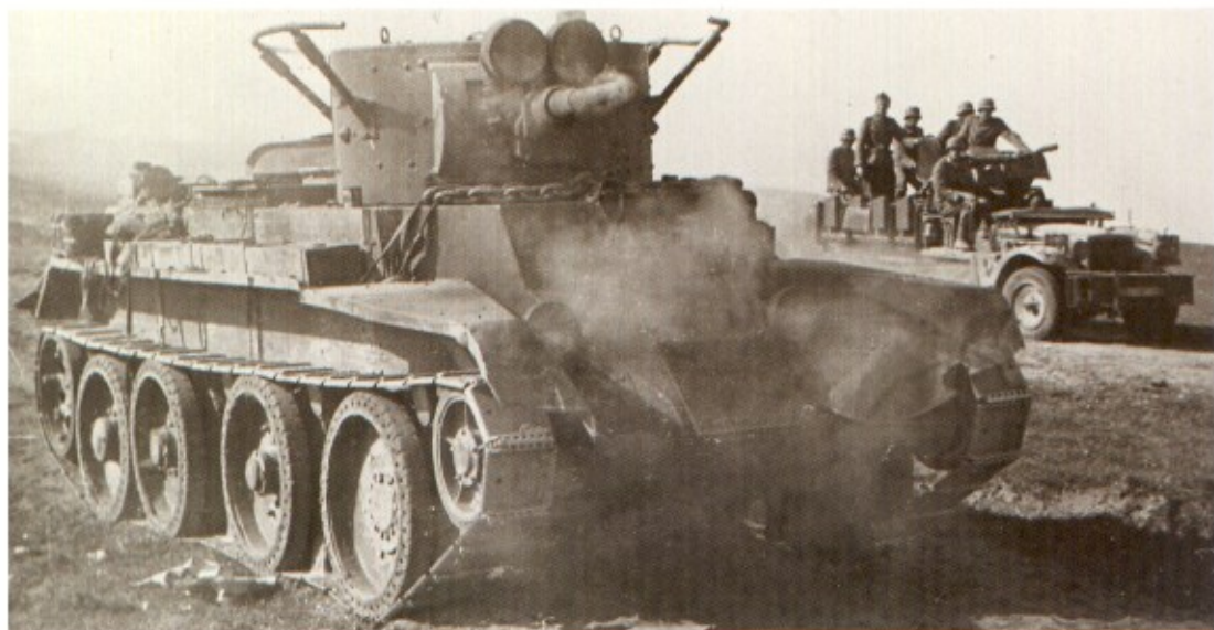
Right: The Commander's version of the BT-7-V was fitted with a very conspicuous frame aerial around the top of the BT-5(V) turret. In the background are German troops on board an Einheits Lkw 6x6 truck. (TM)
