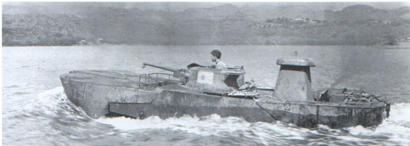
Above and left: Amphibious Tank Type-3 KA-CHI, was based on the CHE HE medium tank. It weighed nearly 29 tons, complete with detachable pontoons. This captured Type-3 is crewed by American servicemen. (TM)
