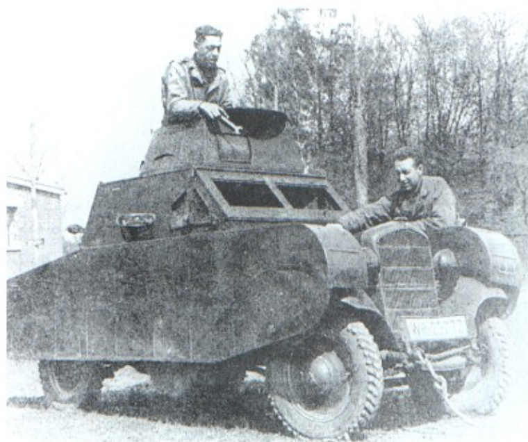
Above: Between the wars the Germans used civilian cars (Dixi/Adler/NSU) fitted with canvas and wood 'tank' bodies for training purposes. (TM)
