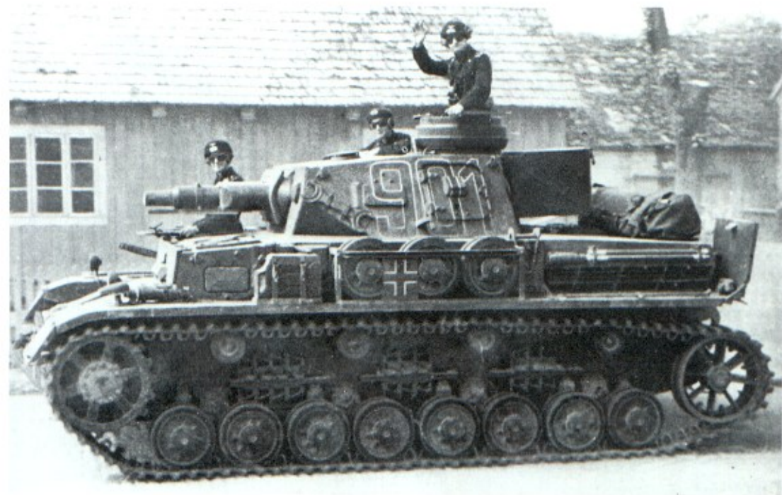
Left: Three of the five-man crew of this PzKpfw IV Ausf D are visible, there remains just the driver and gunner inside. The vehicle number ends in 1, denoting it as the company commander's tank. (TM)
