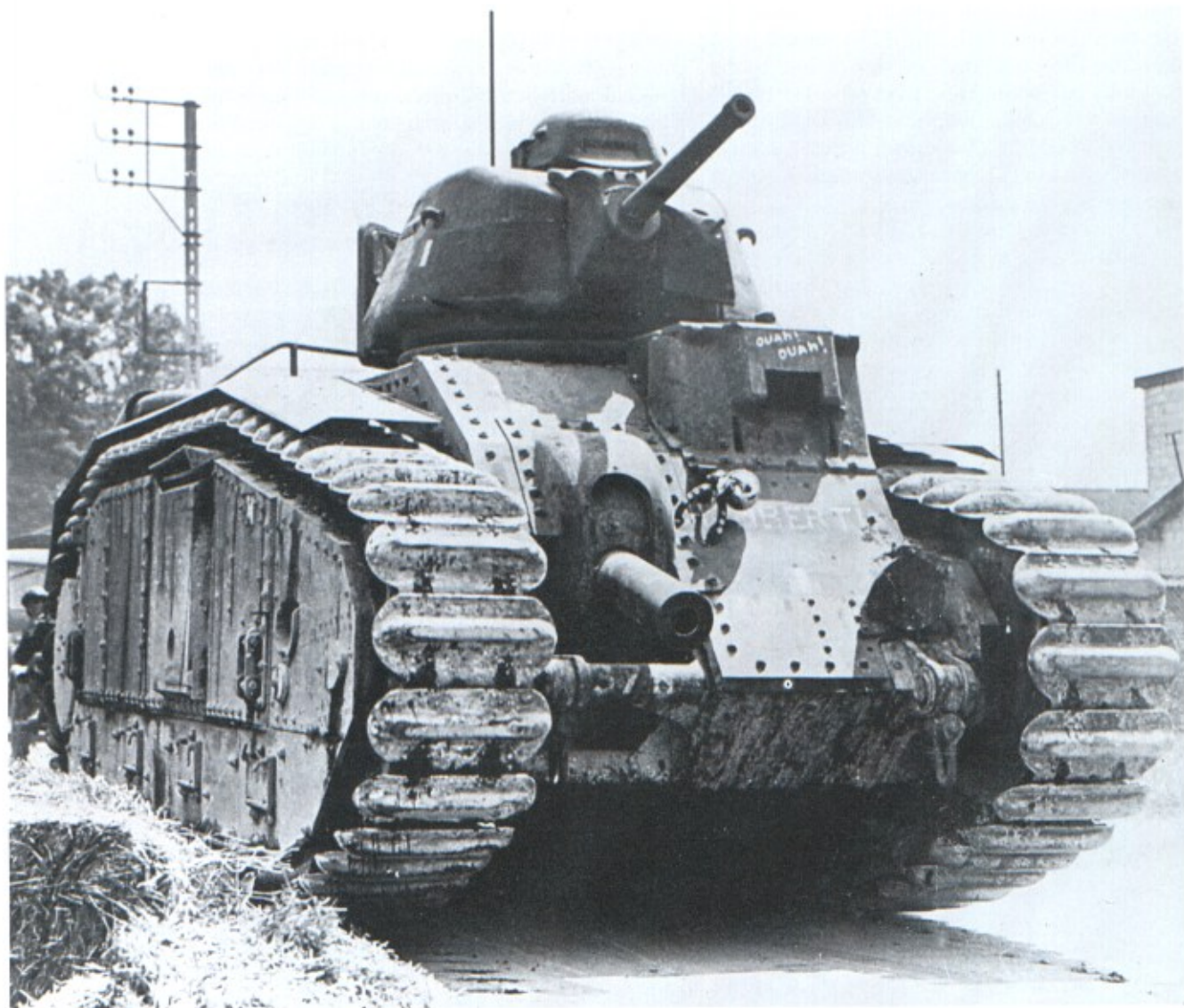
Right: The Char 2C Char du Rupture, was designed in World War One but did not enter service until 1935. The last six of these 68-ton tanks were supposed to have been destroyed by enemy air attack on the way to the front line in May, 1940. This is one of those tanks being examined by German troops and appears undamaged. (TM)
