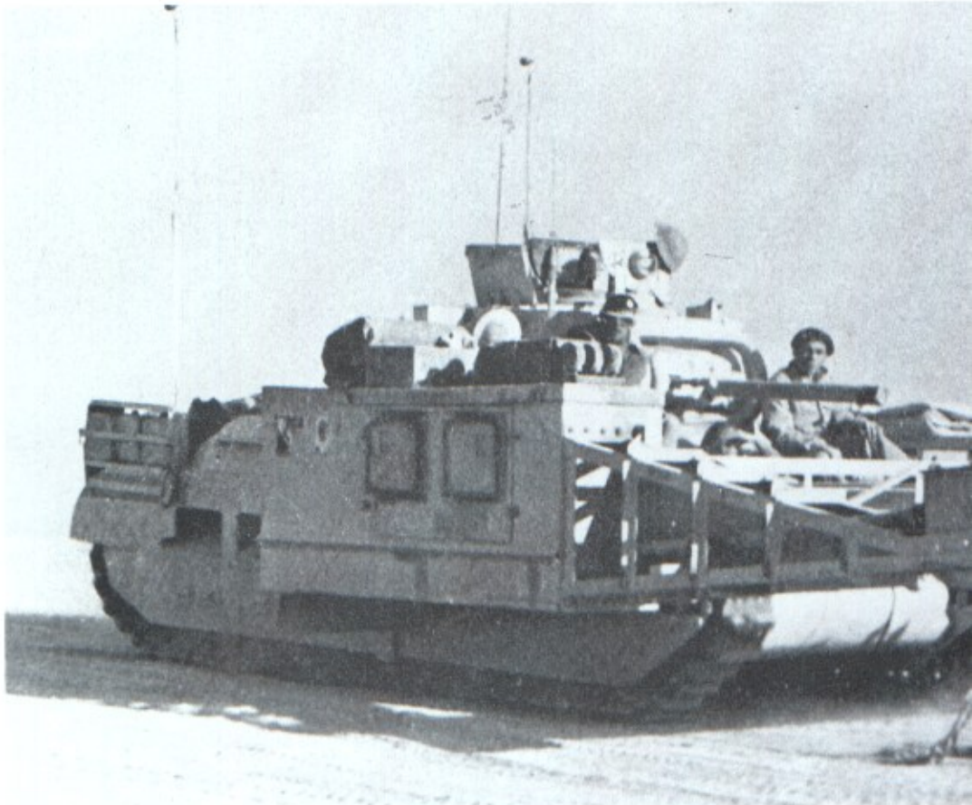
Right: Matilda II equipped with an early Scorpion Mk I mine flail, designed and produced between 1942 and 1943. The drum was driven by a auxiliary engine with the operator seated alongside. The Scorpion Mk II, had better side beams and was operated from inside the tank. (TM)
