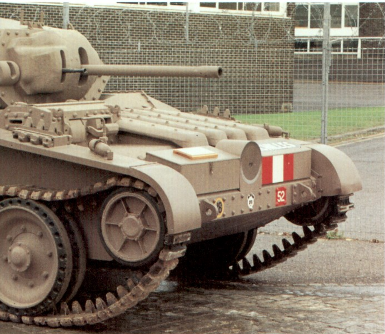
Above: Cruiser Tank Mark V, the Covenanter (A13 Mk III), was a good looking tank with a low silhouette but was a poor performer, being only ever used for training. (TM)
