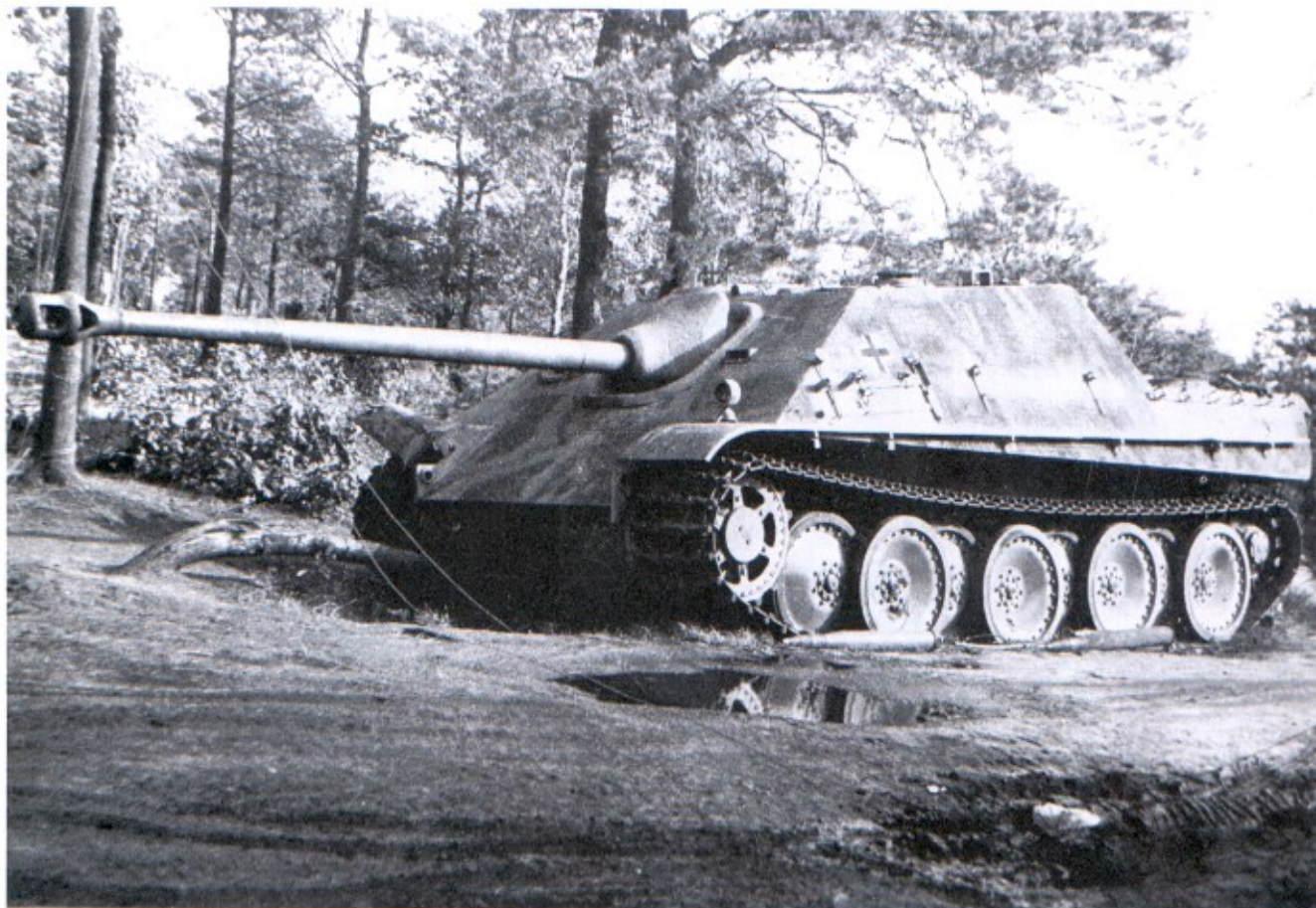
Above: The Jagdpanther was probably the best tank destroyer of the war. Its 88mm gun, low silhouette (only 9ft high) and powerful engine (top speed nearly 30mph) made it widely feared on the battlefield. Less than 400 were built. (TM)
