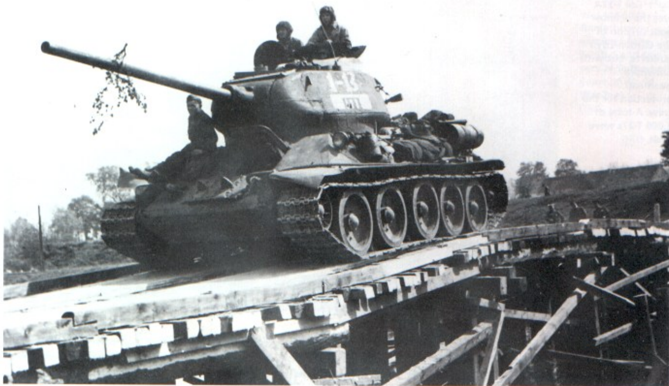
Above: A T-34/85 crosses a temporary bridge on its way to Berlin. This up-gunned version of T-34 was introduced from 1944 onwards. (GF)
