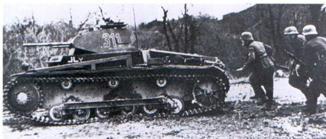
Right: A PzKpfw II Ausf b heading infantry into action. This model and the earlier Ausf a/1, a/2 & a/3 all saw action in Poland as main battle tanks, but were later relegated to the reconnaissance role. (TM)
