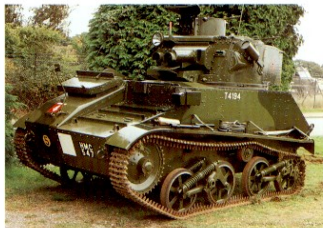
Top: The 13.5 ton Vickers Medium Mk II* was the standard tank of the prewar RTC. (TM)
