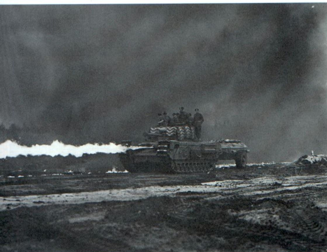
Left: The Churchill flamethrower (Crocodile) was one of the best of its type in the world. Flame fuel was carried in a jettisonable trailer. It could fire 80, one second bursts up to a distance of between 80 and 120 yards. This photograph was taken near Belsen, Germany 1945. (TM)
