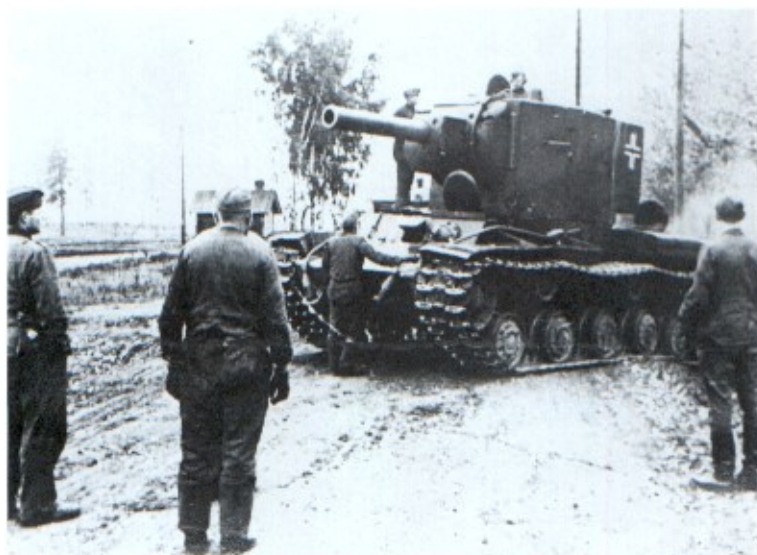
Below: The KV-2A was the close support version mounting a 152mm howitzer in a large, slab-sided turret. It weighed 53 tons. (TM)
