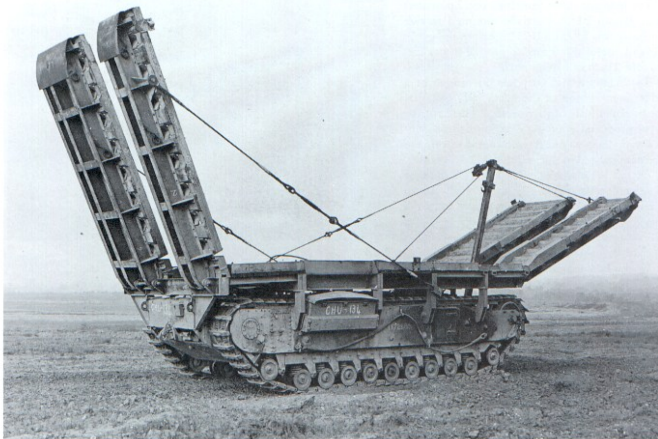
Above Churchill ARK Mk II (British pattern) with ramps raised. The ramps and kingposts were longer than those on ARK Mk I. (TM)
