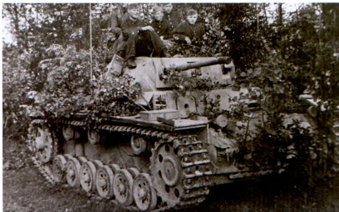
Right: The PzKpfw III Artillerie-Panzerbeobachtungswagen (armoured artillery OP) used a gun tank chassis without turret armament – the dummy gun and centrally-placed machine gun were mounted on a thicker mantlet, the lower MG was also removed. (TM)
