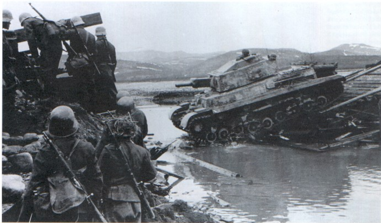
Above: The Hungarian-built Turan II, mounting a very good 75mm gun. Photographed probably in Russia, where the 1st Pancelos Hadosztaly (Hungarian Panzer Division) fought on the Don front, 1943. (TM)
