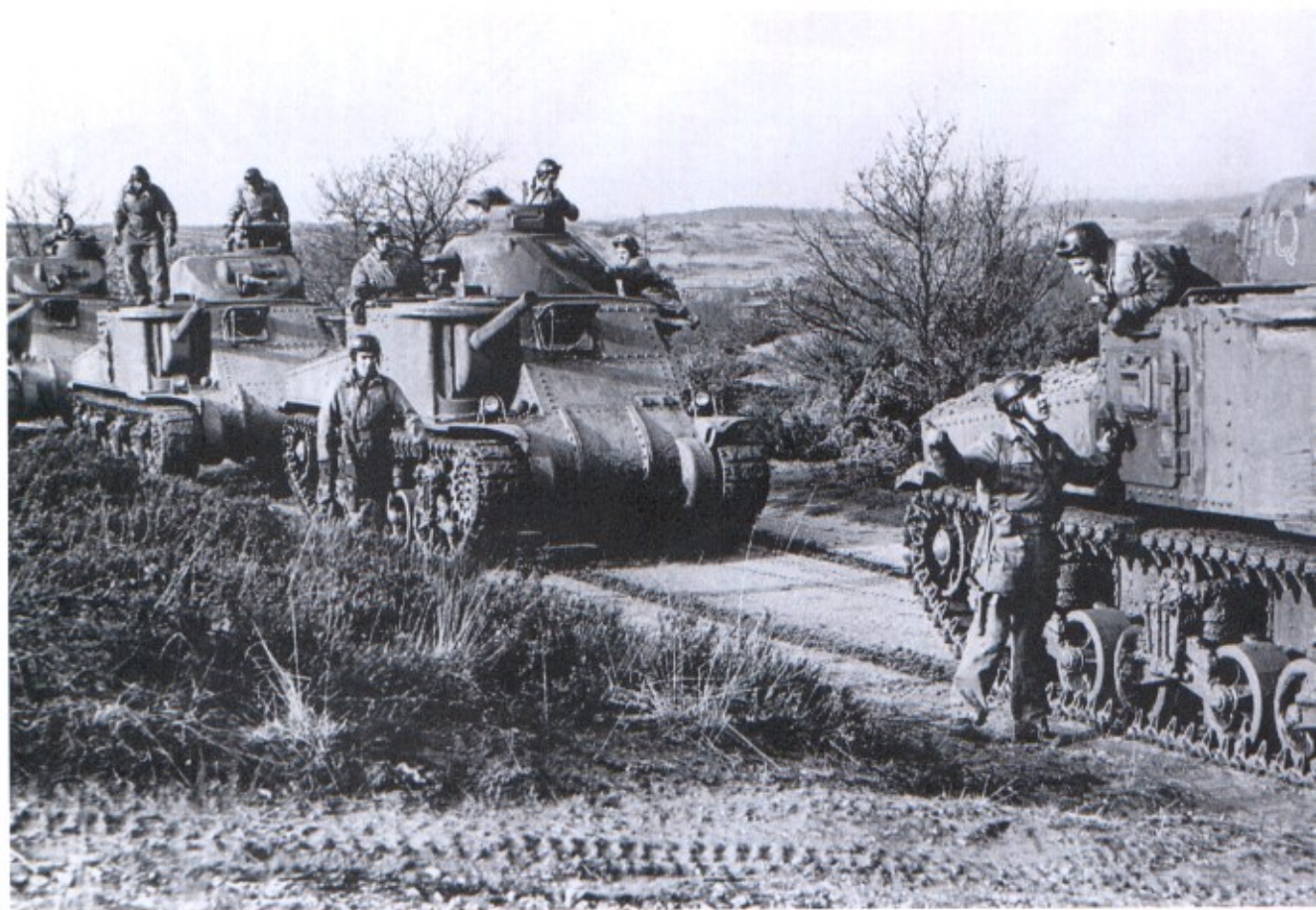
Above: A column of M3 medium tanks on training in Britain. These are the General Lee version, with the commander's cupola, rivetted hull, side doors and powered by a Wright radial engine. They first entered service in April 1941. (TM)
