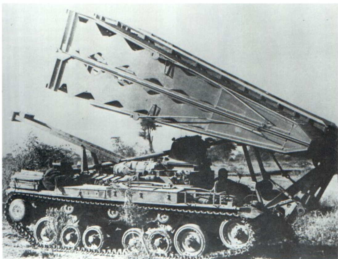
Left: A Valentine bridgelayer about to launch the 30ft scissors-type bridge. Later Valentines were replaced by the Churchill bridgelayer, although some were used in Burma. (T.M.)
