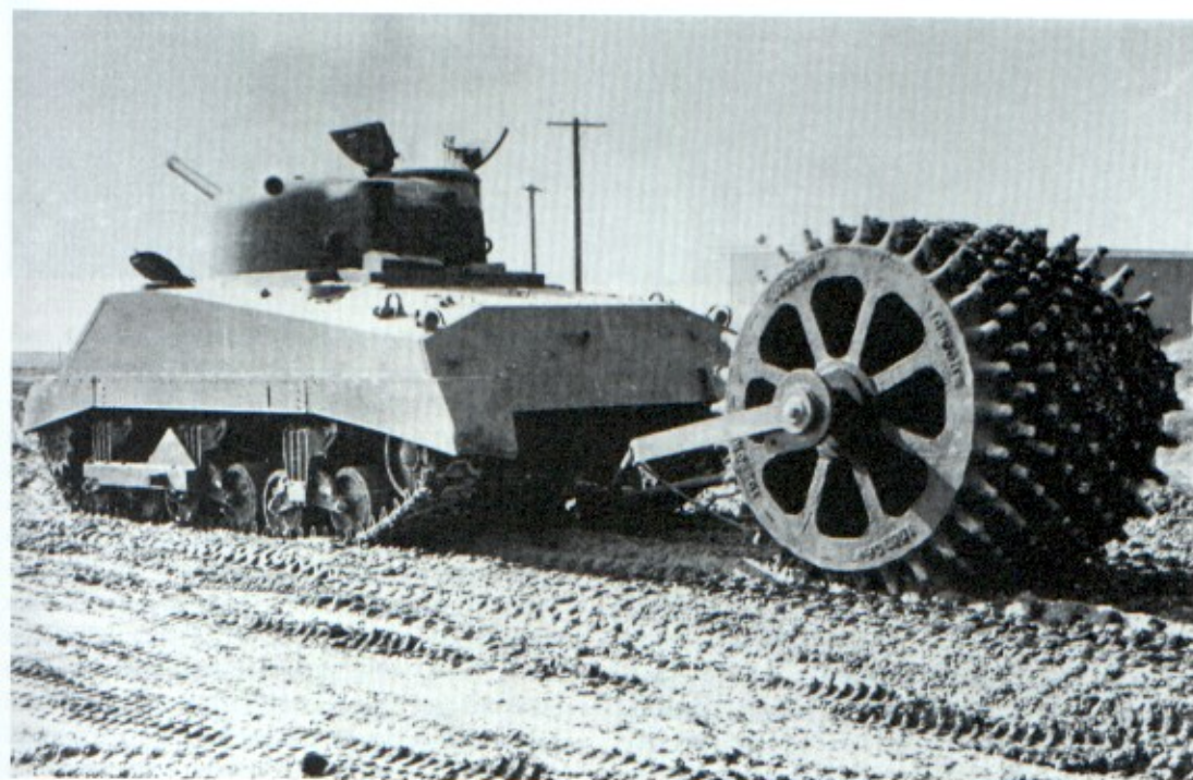
Left: A Sherman T9 mine exploder towing its heavy roller - in action of course it would have been pushed in front to explode the mines. (TM)
