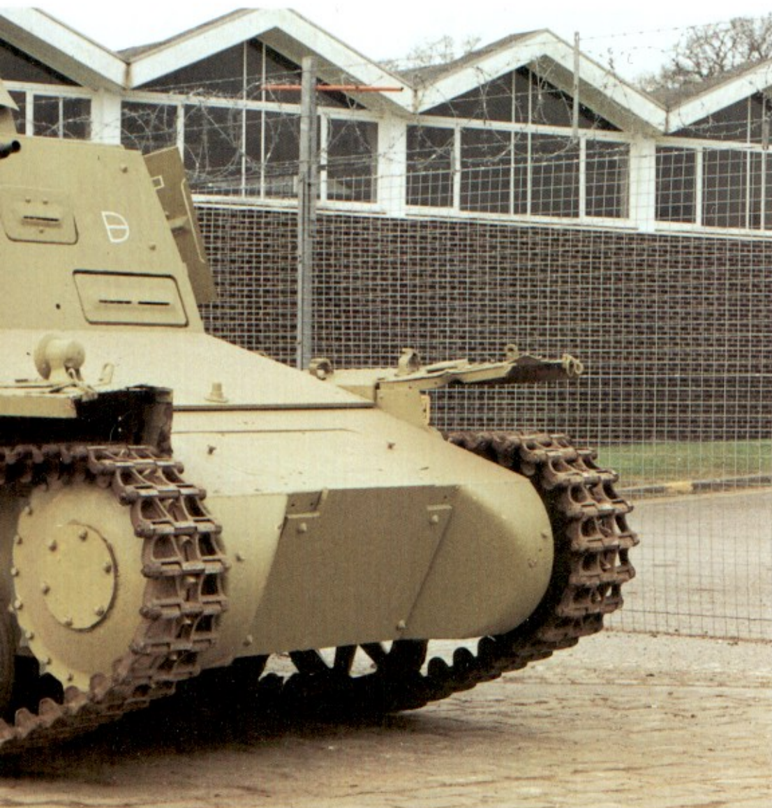
Left: The Kleiner Panzerbefehls-wagen was developed specifically as an armoured command vehicle, based on the PzKpfw I Ausf B. This Kl Pz Bef Wg served with the Deutsches Afrika Korps between 1941-42, was captured in the desert, taken to Britain and inspected in detail at Farnborough in 1943. (TM)
