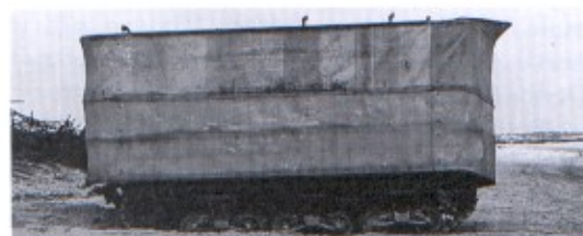
Right: Invented by Nicholas Straussler the Duplex Drive (DD) for amphibious tanks, incorporated a collapsible canvas screen to turn the tank into a boat. Two small swivelling propellers allowed steering, whilst the tracks rotating assisted forward propulsion. Used very successfully by the British on D-Day. (TM)
