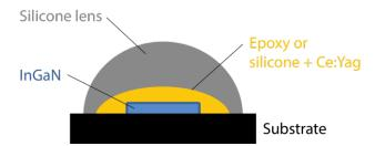
Figure 1: Simplified structure of a white phosphor-coated LED. Source: adapted from [1].
