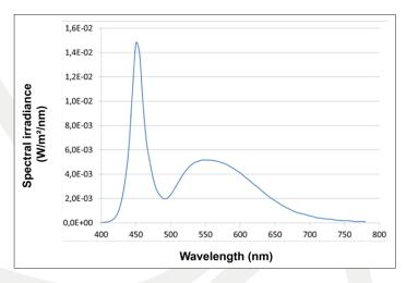
Figure 2: Typical spectrum of a white phosphor-coated LED. Source: adapted from [1].
