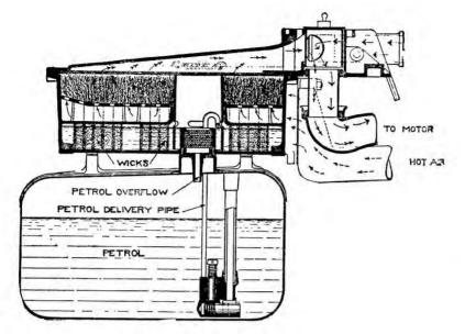
Figure 2. Lanchester Wick Carburettor.
