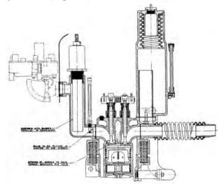
Figure 9. CFR Engine Modifications.
