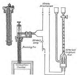
Figure 4. Original Bouncing Pin Knock Detection Equipment.<sup>20</sup>
