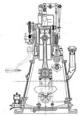
Figure 3. Variable Compression Ratio CFR Engine.<sup>19</sup>
