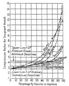
Figure 6. Detonation Characteristics of some Antiknock Standards.
