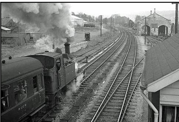
"Railcar" leaving Burdett Road Station in direction of Stroud. A separate steam engine was attached to the carriage from well before WWII. Goods shed and signal box on right; brickworks on left.
