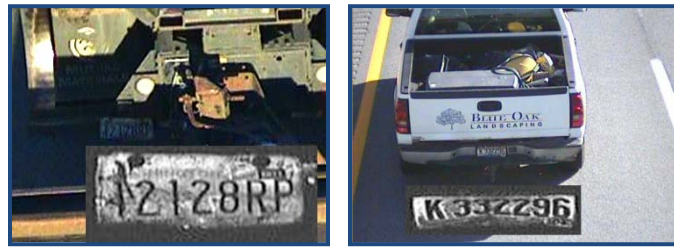
Figure 11: Bent, Dirty, or Damaged Plates
