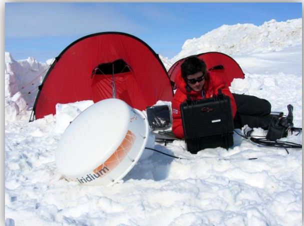
Fig. 5.2. Communicating from the Field with the Iridium OpenPort System. Source: Arctic Jubilee Expedition 2012.
