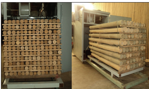
Photo 1. Stacking basic parts of T. siamensis and middle parts of D. asper
