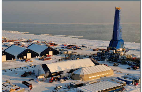
On Sakhalin Island, the Yastreb rig is drilling extended-reach development wells 6 miles into the offshore Odoptu field from the onshore location pictured below.
