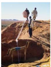
Fig. 3: While a man works at the bottom of the 18m shaft his partners keep the oxygen flowing.
