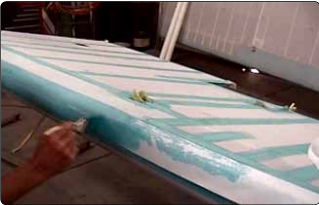
Figure 3-33. Cement is brushed through a four-inch tape during installation over the fabric seam on a wing leading edge. Two-inch tapes cover the wing ribs and rib lacing.
