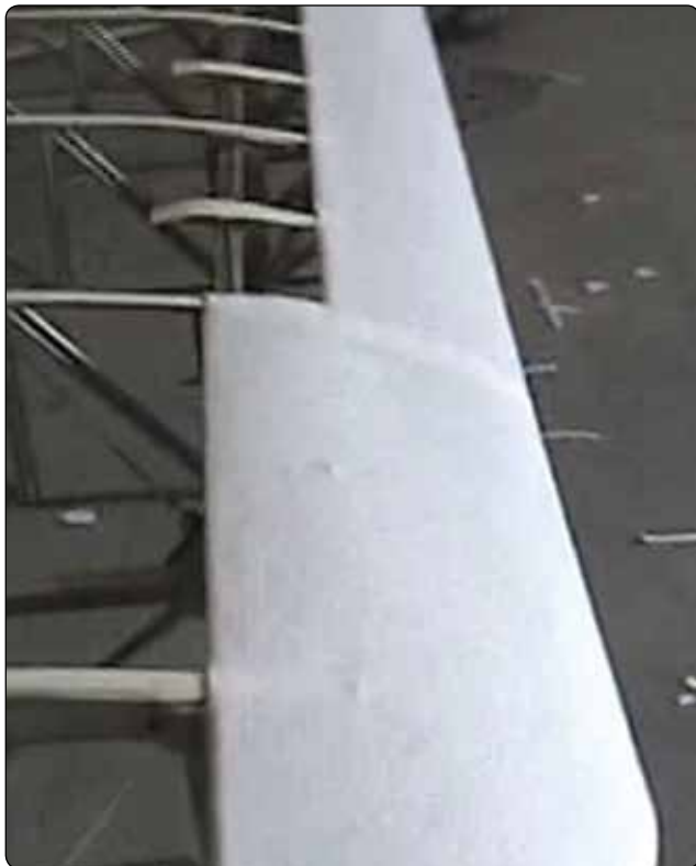
Figure 3-17. The use of specified felt or padding over the wing leading edges before the fabric is installed results in a smooth regular surface.
