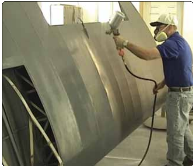
Figure 3-34. Applying a primer with UV blocking by spraying cross coats.
