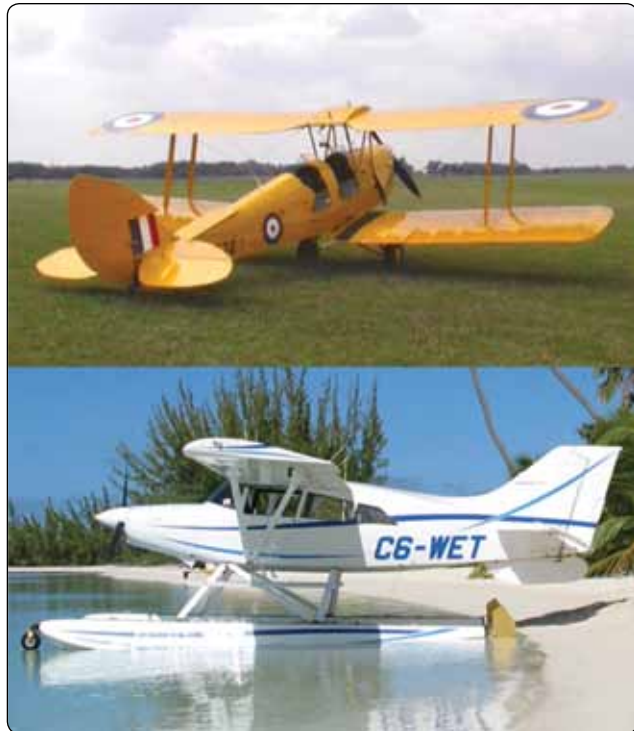
Figure 3-1. Examples of aircraft produced using fabric skin.
