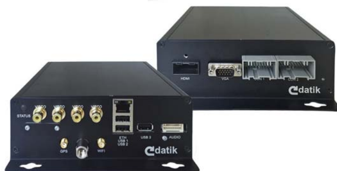
Figure 3: System design example for faster upgrades: Datik's DCB fleet edge computer is equipped with i.MX6-based Qseven Computer-on-Modules from congatec, which can easily be swapped for the even more powerful new i.MX8 performance class modules.
