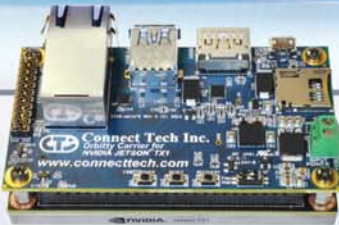
Orbitty Carrier for NVIDIA® Jetson™ TX2 or TX1
