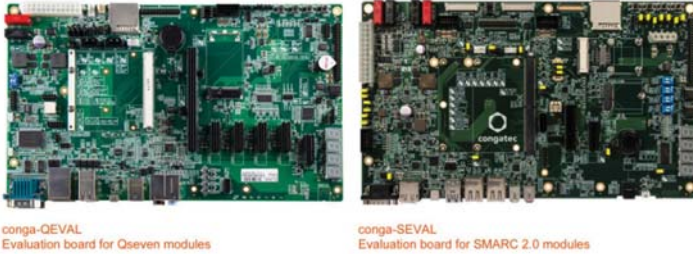
Figure 4: Evaluation boards for Computer-on-Modules provide an essential basis for OEMs' own carrier board designs.
