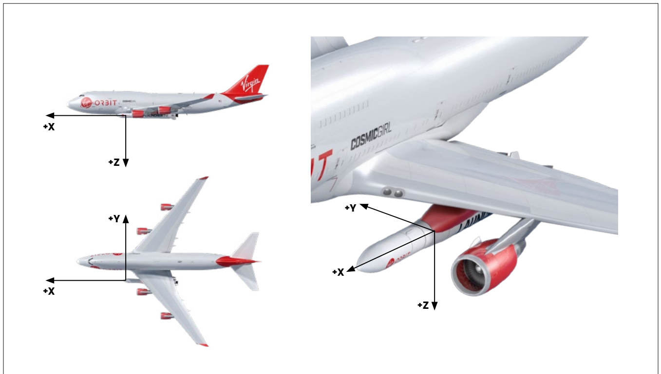
FIGURE 11/ LAUNCH VEHICLE COORDINATE SYSTEM
