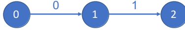
Figure 6.5: Multibody system with three rigid bodies and two joints in a straight chain.
