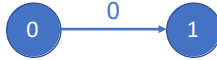
Figure 6.4: Kinematic pair with two rigid bodies (vertices 0, 1) that are connected via a joint (edge 0).
