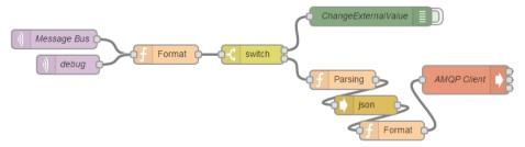
Figure 4: Notification output towards ReactiveBox application system (AMQP protocol)
