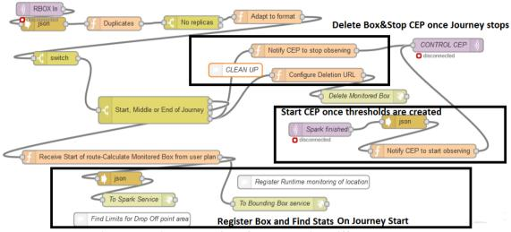
Figure 7: Middleware flow for connecting different layers
