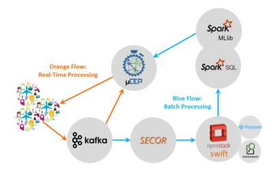
Figure 3: Information Lifecycle Management flow (orange is real-time flow, blue is ingestion and analysis flow)
