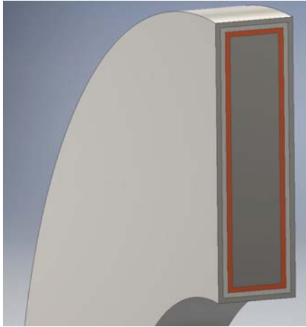
Figure 39. Cross-Section of a Coil showing copper sheathing (for current transients) and structural shell
